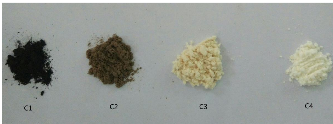
Fig. 5. Appearance of crude cellulose separated by various DESs (140 °C for 90 min) (C1) DES1, (C2) DES2, (C3) DES3, and (C4) DES4
