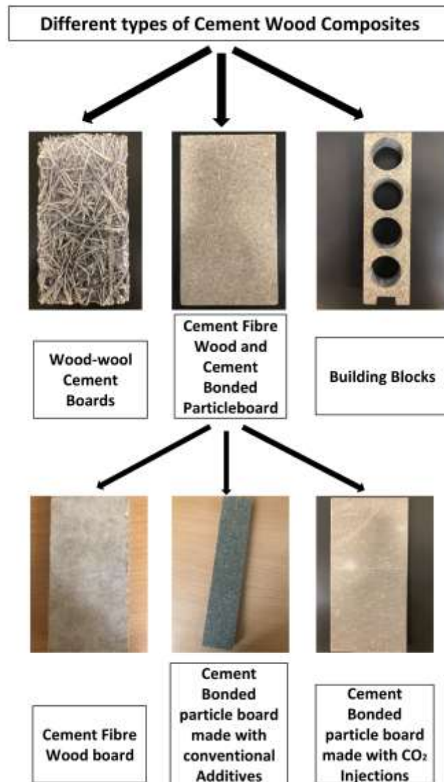
Fig. 1. Schematic diagram of different types of Cement Wood Composites (CWC)
