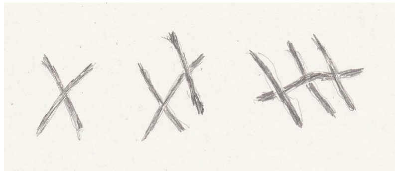
Fig. 1. Illustration of fibre contacts for various values of N : (a) Occasional contact ( N = 1 ); (b) Connectivity threshold ( N = 16 ); (c) Rigidity threshold ( N = 60 )
