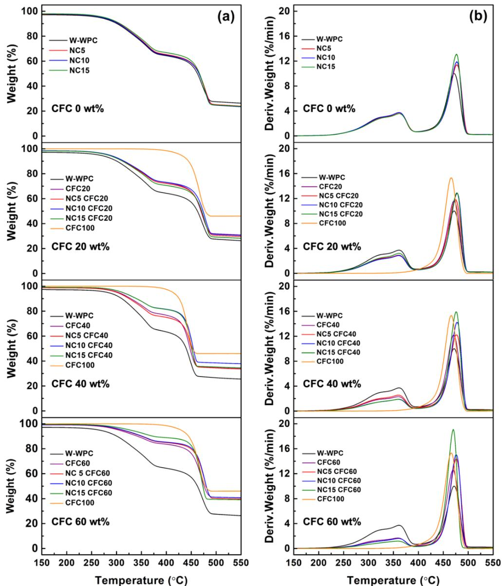
**Fig. 6.** TGA properties of recycled WPCs filled with carbon fiber and nanoclay: (a) TG curves, (b) DTG curves
