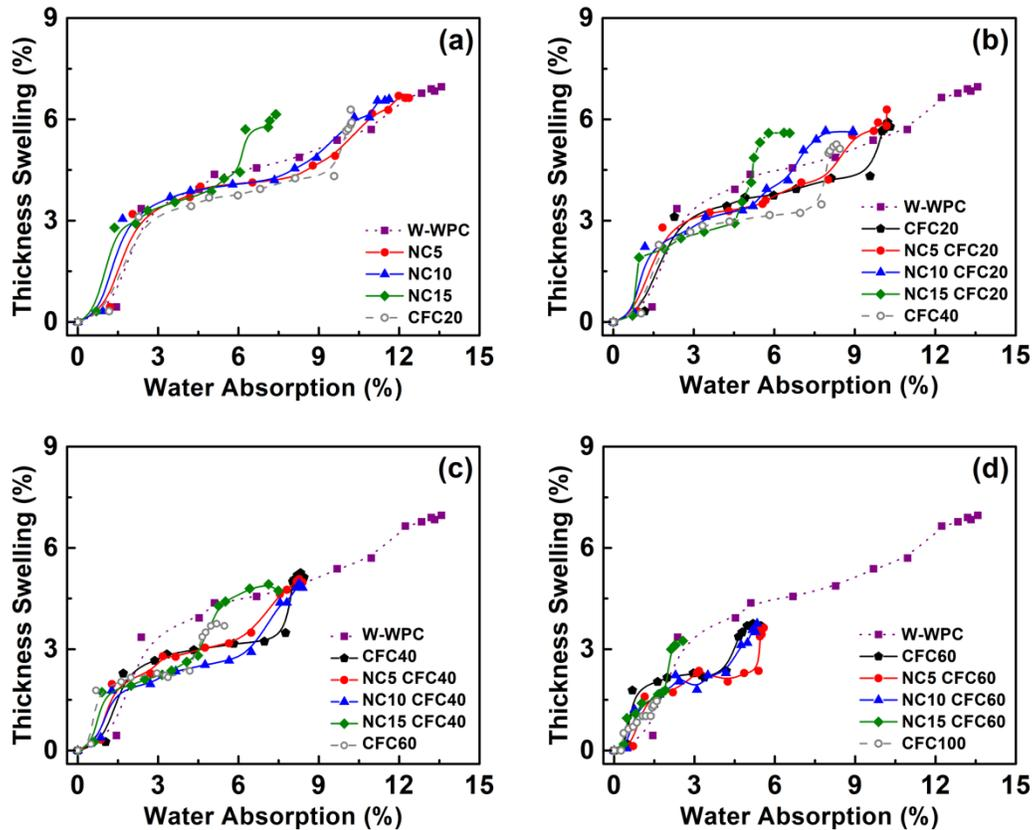
**Fig. 7.** Water absorption and thickness swelling curves of recycled WPCs filled with carbon fiber and nanoclay: (a) CFC 0 series, (b) CFC 20 series, (c) CFC 40 series, and (d) CFC 60 series
