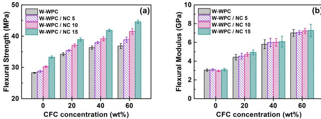
**Fig. 5.** Flexural properties of recycled WPCs filled with carbon fiber and nanoclay: (a) flexural strength and (b) flexural modulus
