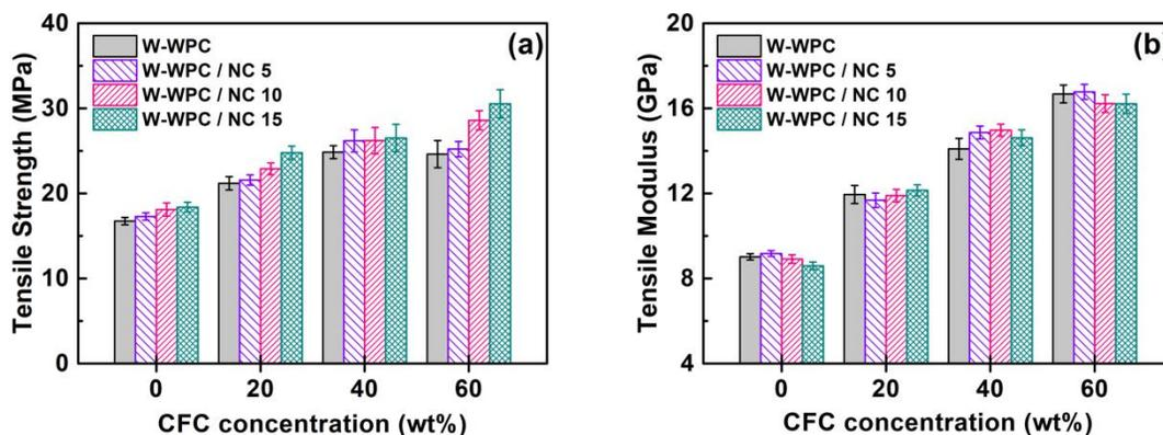
**Fig. 4.** Tensile properties of recycled WPCs filled with carbon fiber and nanoclay: (a) tensile strength and (b) tensile modulus
