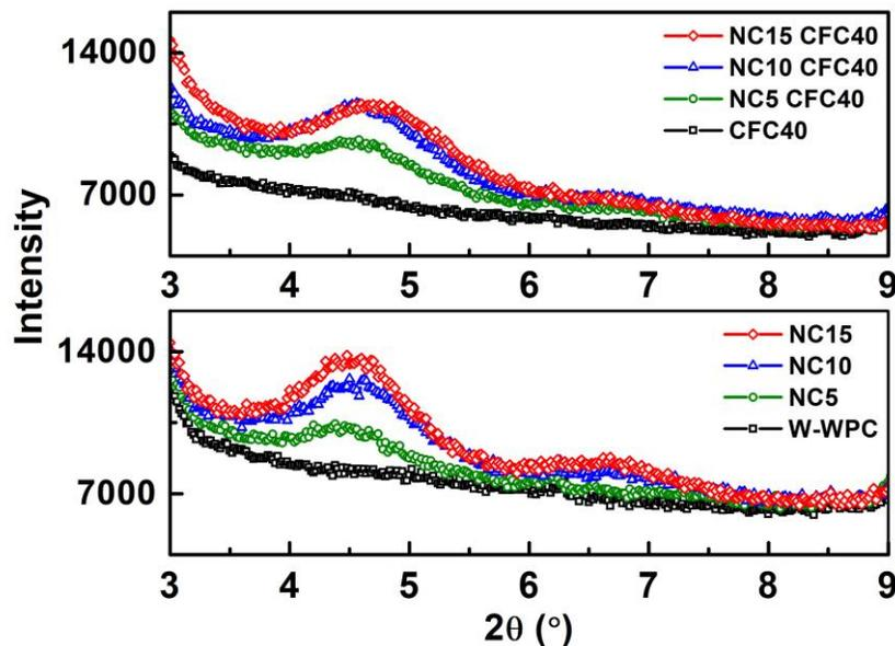
Fig. 1. The XRD patterns of recycled WPCs filled with carbon fiber and nanoclay
