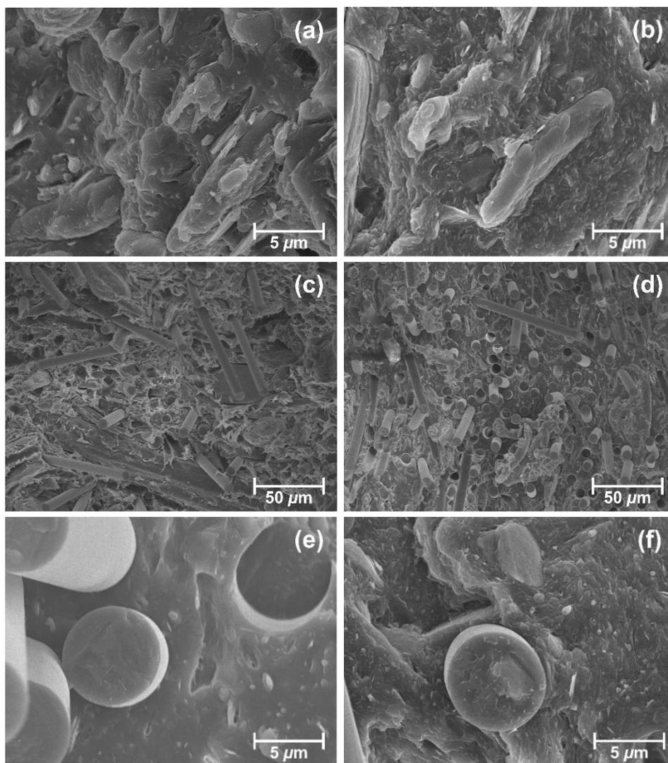
**Fig. 2.** The SEM images of the impact-fractured surfaces of recycled WPCs filled with carbon fiber and nanoclay: (a) W-WPC (5000 $\times$ ), (b) NC15 (5000 $\times$ ), (c) CFC20 (500 $\times$ ), (d) CFC60 (500 $\times$ ), (e) CFC60 (5000 $\times$ ), and (f) NC15 CFC60 (5000 $\times$ )
