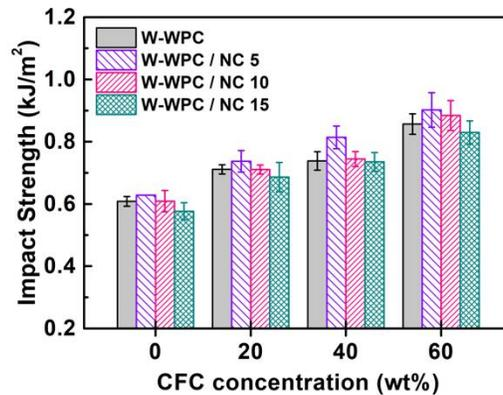
**Fig. 3.** Impact strength of recycled WPCs filled with carbon fiber and nanoclay
