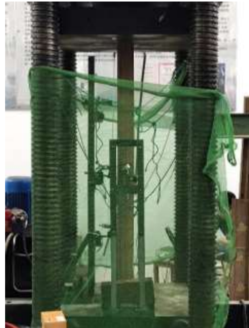
Fig. 4. The test device used for axial compression testing
