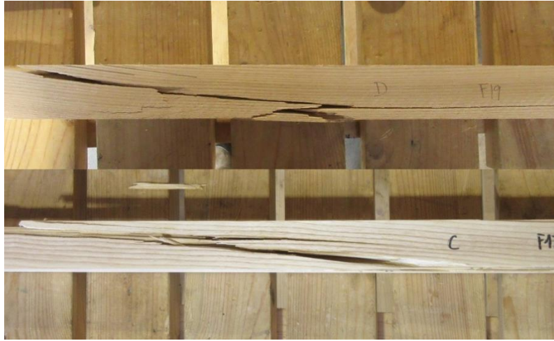
Fig. 5. The failure patterns following the ring boundaries on radially sawn white ash specimens
