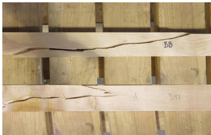
Fig. 4. Wavy-grained yellow birch specimens after failure
