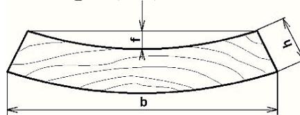
**Fig. 8.** Diagram of measured parameters for determining cross warping
