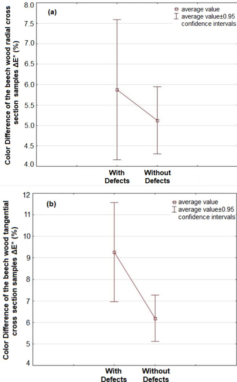
**Fig. 10.** Average values and confidence intervals of color difference parameters ( $\Delta E^*$ ) of the beech wood with defects and without defects: (a) radial cross section samples and (b) tangential cross section samples
