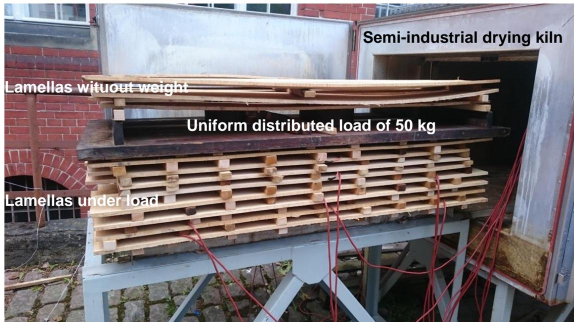
**Fig. 4.** View of the drying kiln and lamellas' stack before drying process
