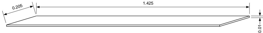
**Fig. 3.** The main dimensions (in m) of the wood lamellas prepared for the drying process
