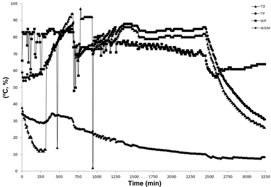
**Fig. 7.** The variable changes during the beech wood drying process: TD – wood temperature (°C); TP – drying medium temperature (°C); WP – drying medium humidity (%); and WDM – wood moisture content (%)
