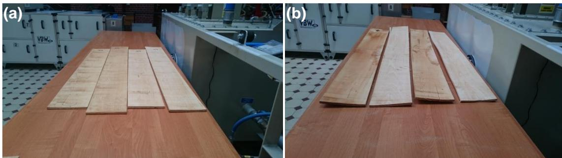
**Fig. 9.** Selected beech wood lamellas after drying process: (a) under load of 50 kg and (b) without load
