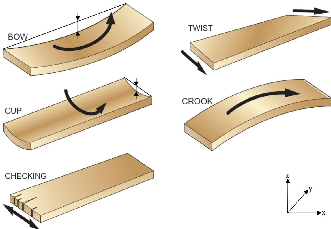
**Fig. 2.** Examples of wood deformations (Permission granted from Woodcraft magazine; Hurst-Wajszczuk 2008)
