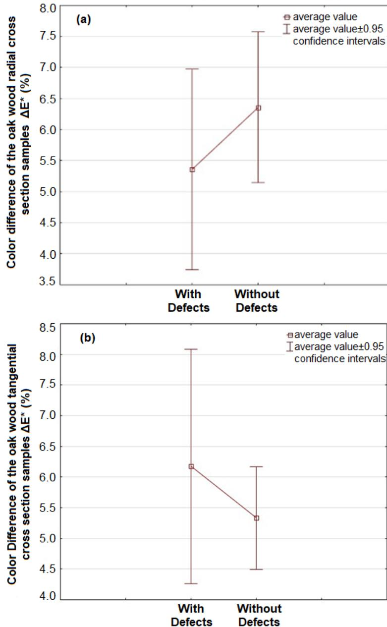
**Fig. 11.** Average values and confidence intervals of color difference parameters ( $\Delta E^*$ ) of the oak wood with defects and without defects: (a) radial cross section samples and (b) tangential cross section samples
