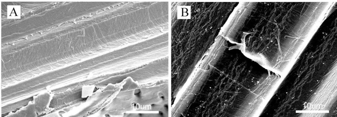
**Fig. 8.** Scanning electron microscopy images of the untreated (a) and dye-treated BFC (b) after 90 days weathering
