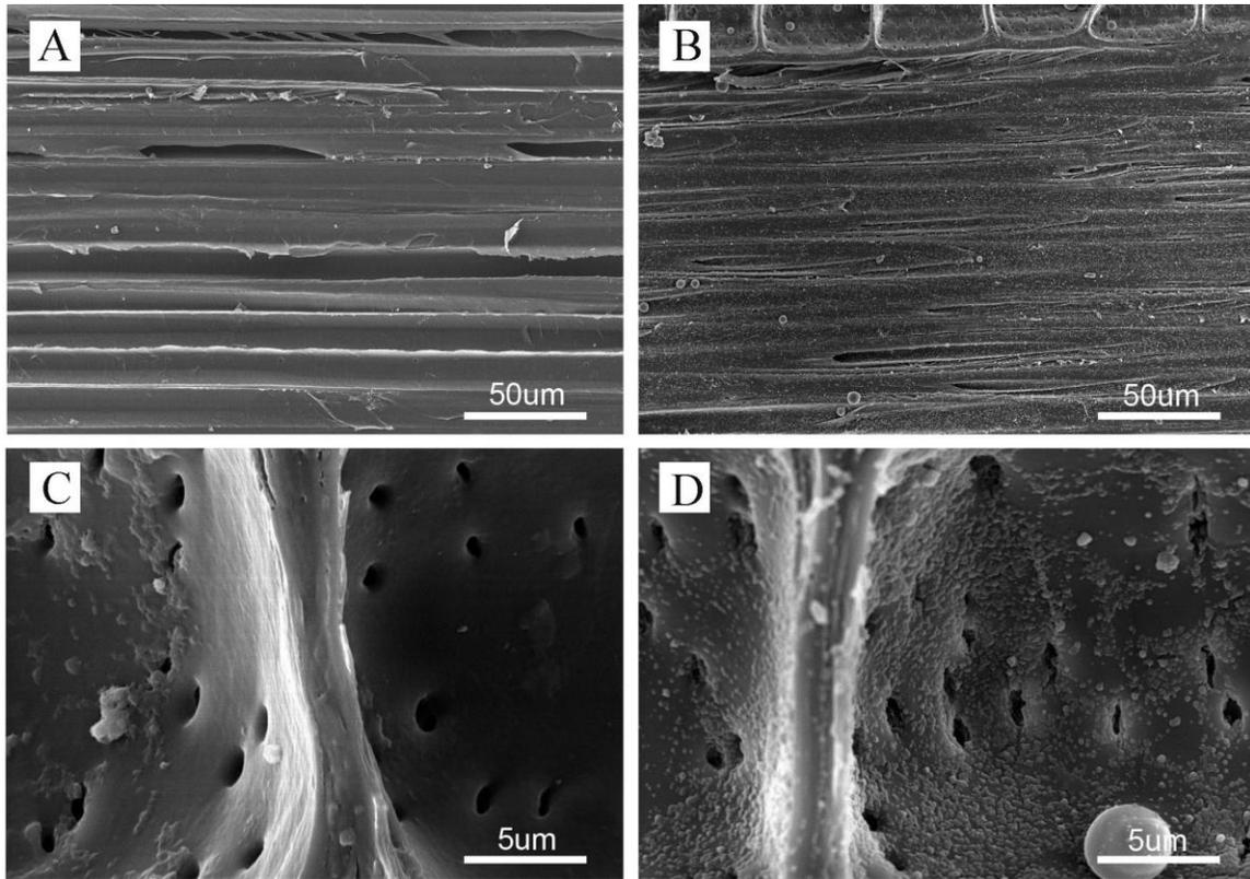
**Fig. 7.** Scanning electron microscopy images of the untreated and dye-treated bamboo fibers
