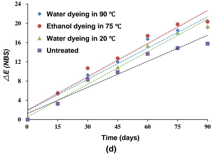
**Fig. 4.** Changes of color parameters of BFC samples during the period of 90 days of outdoor exposure: (a) brightness,  $L^*$ ; (b) red-green spectrum,  $a^*$ ; (c) yellow-blue spectrum,  $b^*$ ; (d) Total color difference ( $\Delta E^*$ ).
