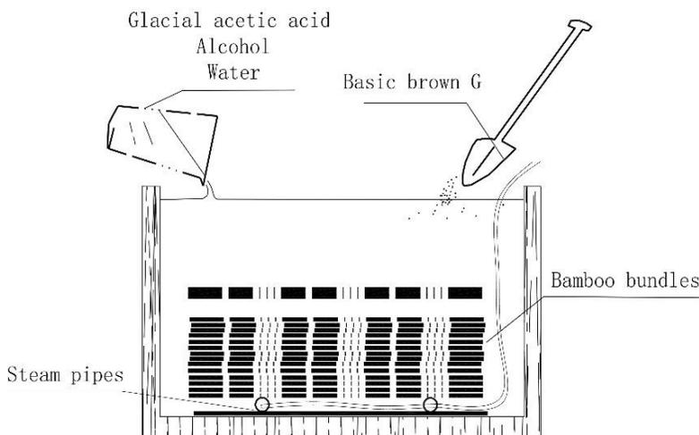
**Fig. 2.** Schematic diagram of dye bath for bamboo fiber bundles.
