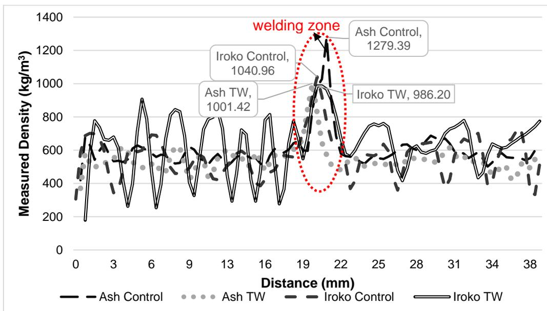
Fig. 4. Measured density profile of Iroko and ash
