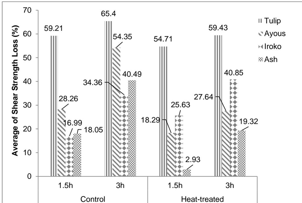
**Fig. 2.** Average of shear strength loss (%)
