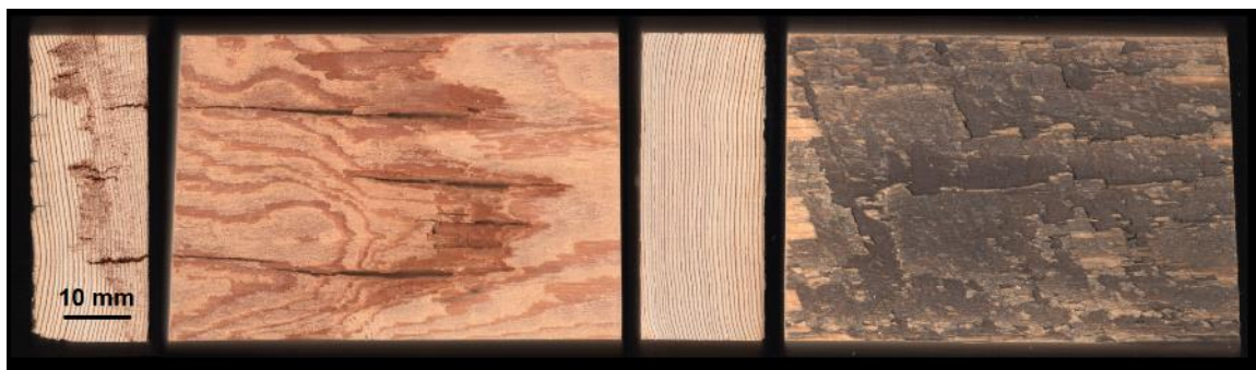
Fig. 5. Example of weathered eastern hemlock ( Tsuga canadensis ) on tangential surface. Left side degraded by fungi due to long-term moisture accumulation; right side exposed to weathering.
