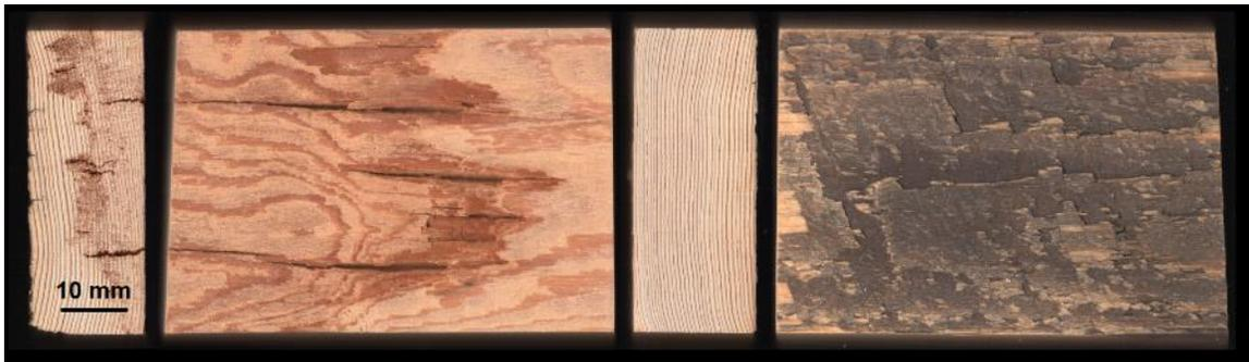
**Fig. 5.** Example of weathered eastern hemlock (*Tsuga canadensis*) on tangential surface. Left side degraded by fungi due to long-term moisture accumulation; right side exposed to weathering.
