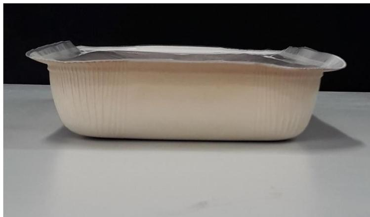
**Fig. 2.** Impact of tray flange distortion on tray width
