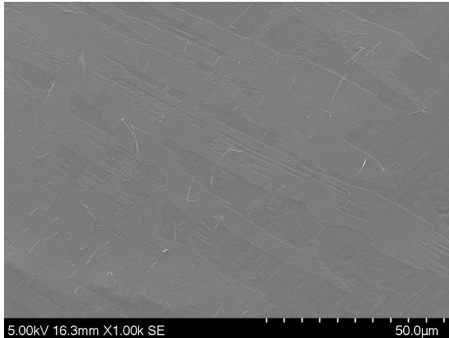
**Fig. 10.** Surface morphology of the PET coating after drying the tray
