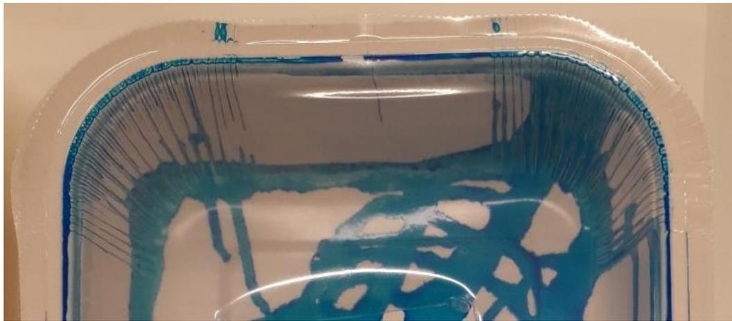
**Fig. 7.** Corner crease leaks on dried trays
