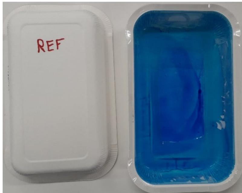
**Fig. 8.** Leak tests of the empty trays before being heated
