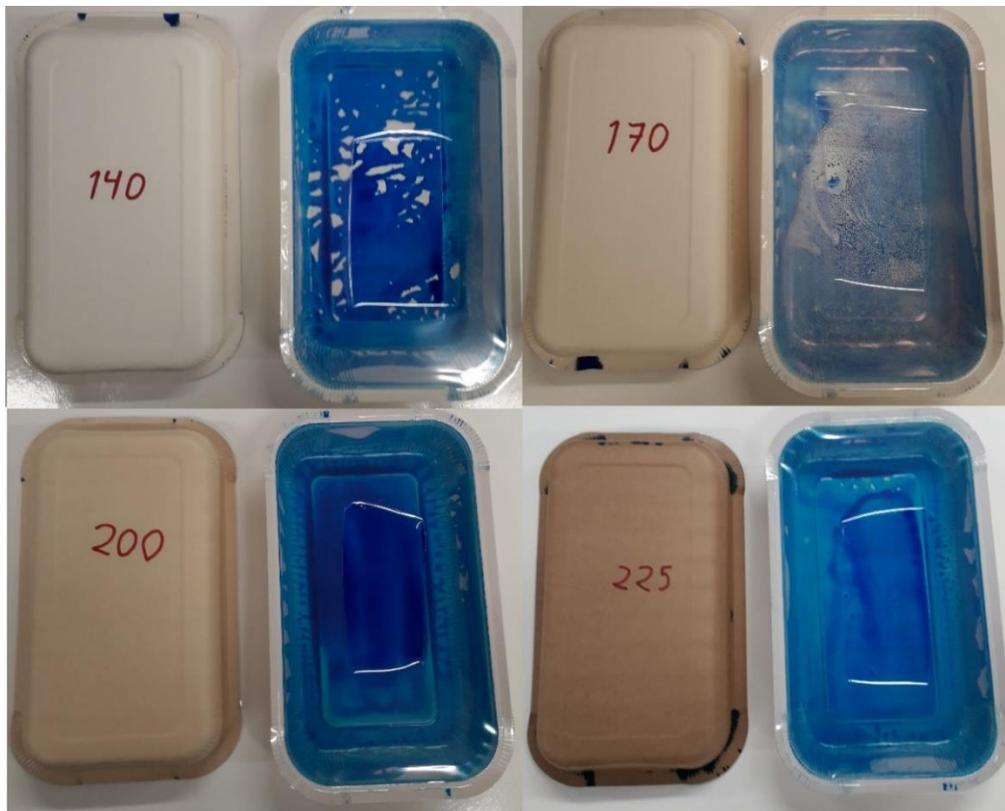
**Fig. 6.** Leak tests after heating the empty trays (indicated heating temperature is in °C)
