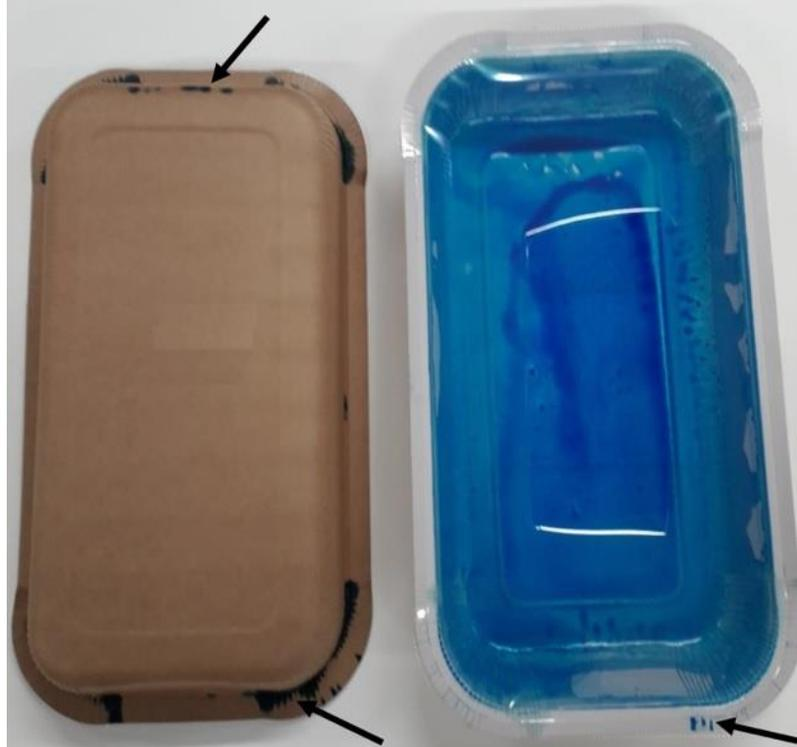
**Fig. 1.** Pinholes (left) and corner creases leaks (right) highlighted with arrows on bottom and top of sealed trays
