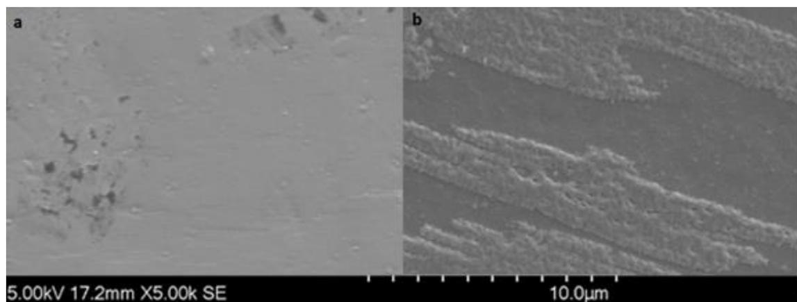
**Fig. 9.** Surface morphology of the PET coating (a) before and (b) after the food processing procedure
