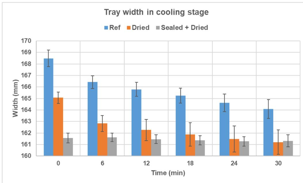
**Fig. 4.** Tray dimension measurements during the cooling stage of the food processing procedure
