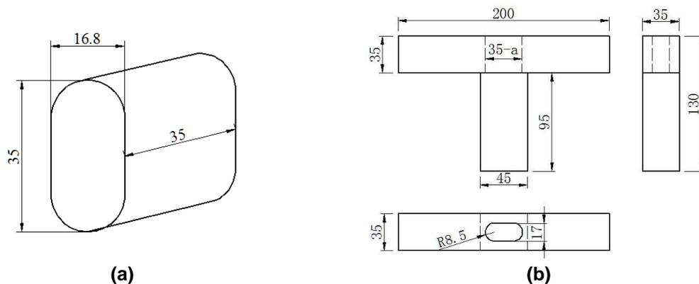
**Fig. 2.** Dimensions of specimens: (a) oval tenon and (b) T-shaped specimen; all units are in mm
