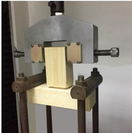
Fig. 5. Setup of measuring withdrawal load resistance
