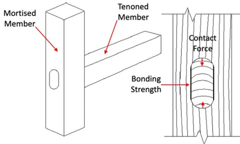
**Fig. 1.** Mechanical analysis of the mortise and tenon joints in actual state
