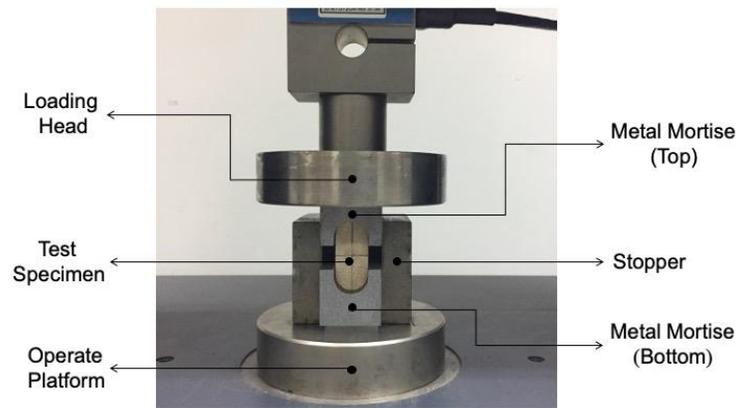
**Fig. 4.** Setup for test method for direct measuring contact force and its relaxation of M-T joints
