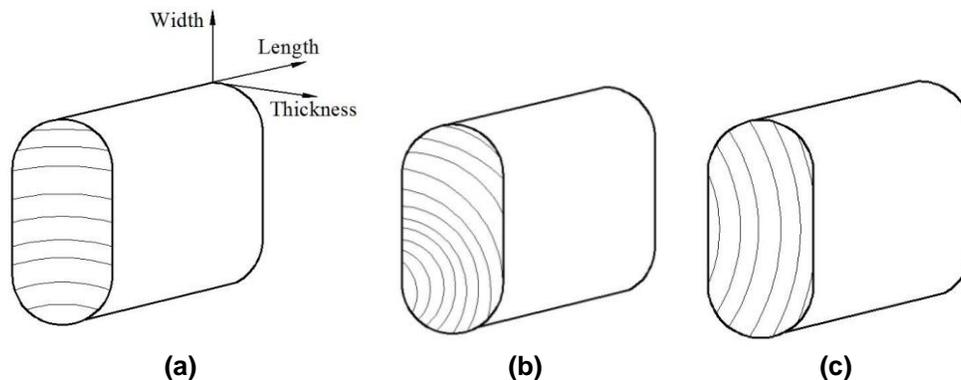
**Fig. 3.** Diagram of wood grain orientation of tenon in its width direction: (a) radial orientation; (b) diagonal orientation; (c) tangential orientation
