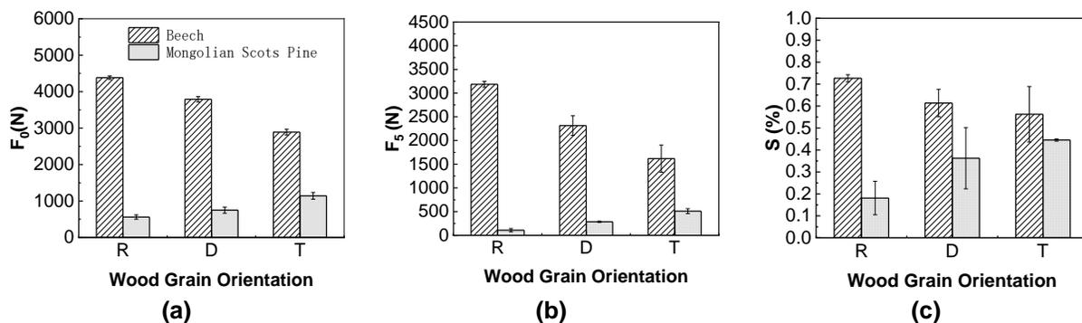
**Fig. 8.** The contact force and its retention of the M-T joints between beech and Mongolian Scots pine wood
