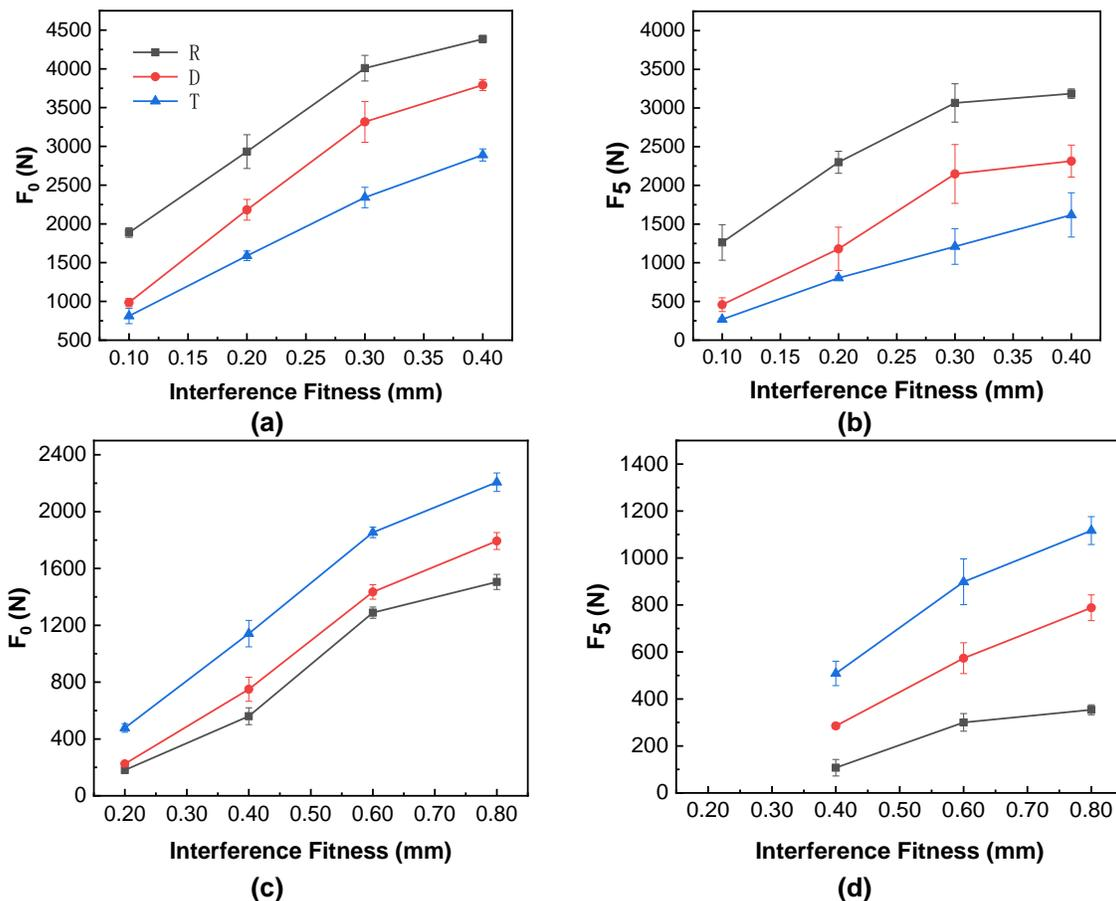
**Fig. 7.** The interference fitness-contact force curves of R, D, and T grain orientation: (a)  $F_0$  of beech wood; (b)  $F_5$  of beech wood; (c)  $F_0$  of pine wood; (d)  $F_5$  of pine wood
