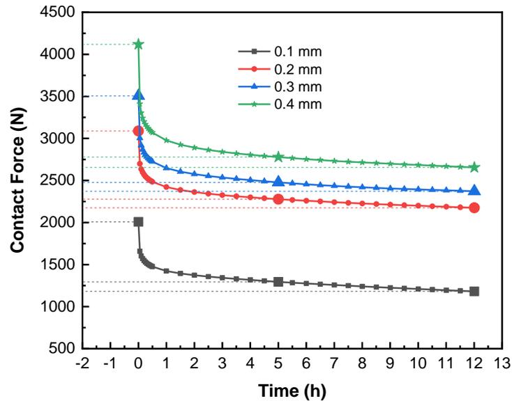
Fig. 6. Relaxation curve of the contact force of the M-T joints after 12 h
