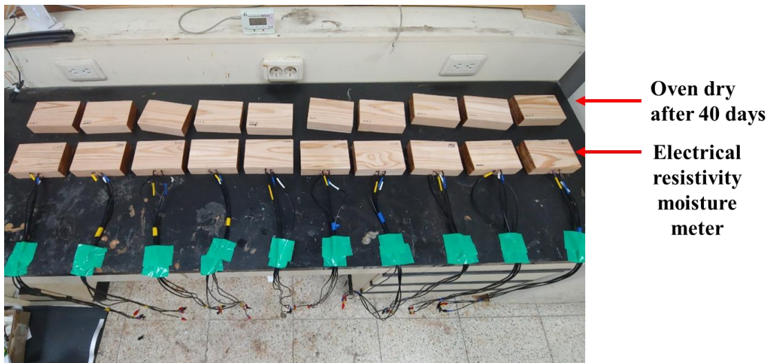
Fig. 3. Preliminary test for the calculation of the calibration moisture content of the electrical resistivity-moisture content measurement method
