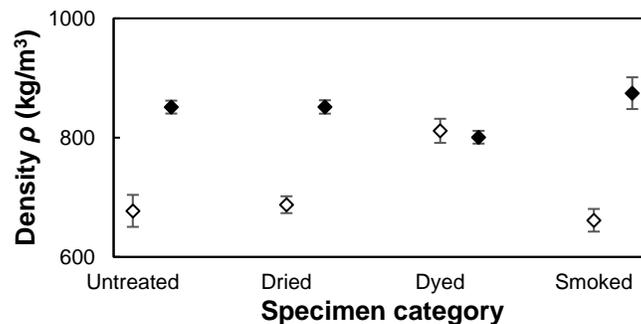
**Fig. 3.** Mean values of density variation in untreated and modified bamboo; Mode A:  $\diamond$   $n = 8$ , Mode B:  $\blacklozenge$   $n = 5$ ; error bars represent the standard deviation
