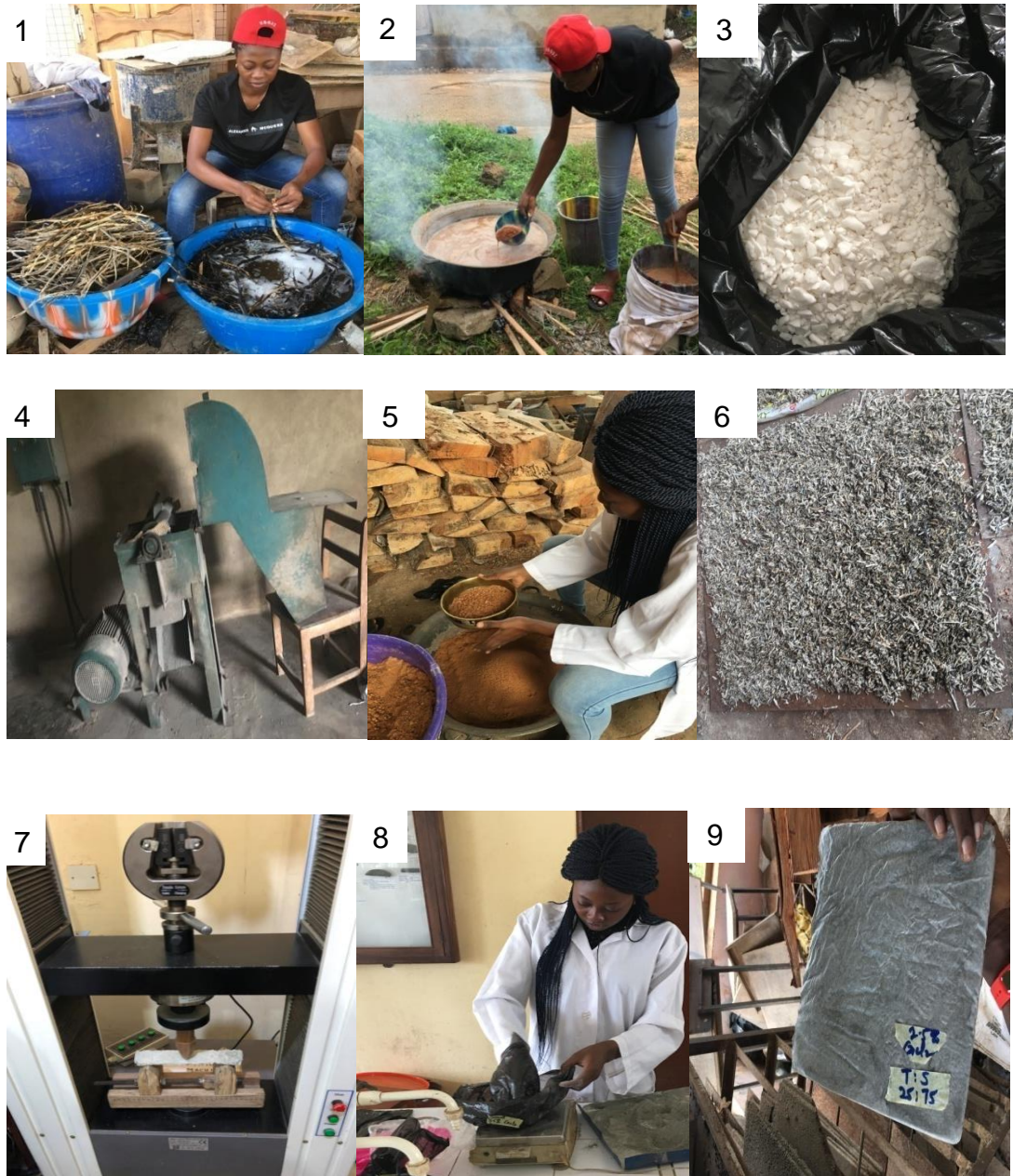
Fig. 1. (1) Cleaning tomato stems; (2) pretreatment of coconut husk dust; (3) additive (calcium chloride); (4) milling machine used to reduce tomato stem and husk size; (5) sieving of coconut husk dust after milling; (6) drying of milled tomato stem particles; (7) sample under test; (8) weighing of board contents; (9) board produced
