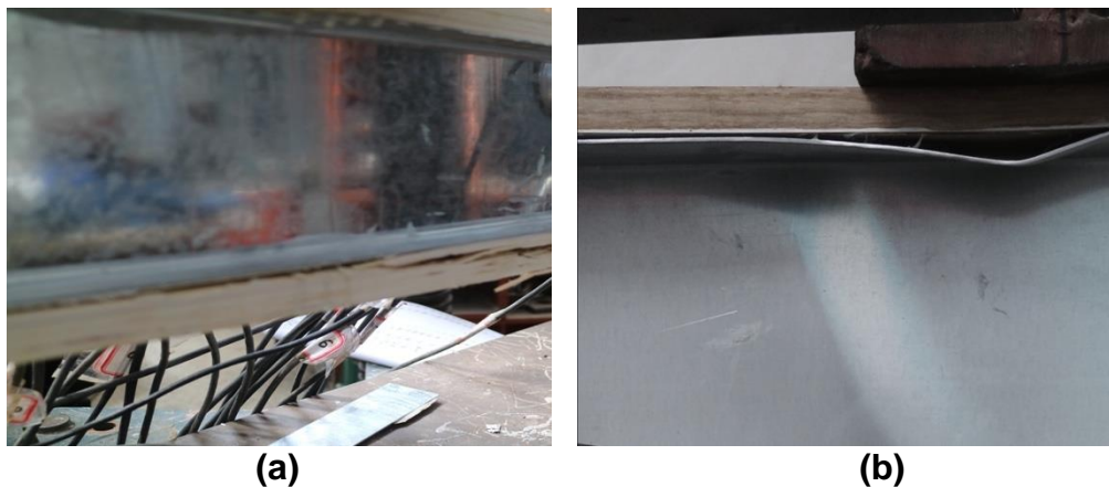
Fig. 6. Failure modes of L-7: (a) the lower flange plywood cracked at mid-span section and (b) the shearing failure of web at the loading point
