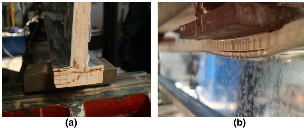
Fig. 5. Failure modes of L-6: (a) the LVL plywood at the lower beam end cracked and (b) the LVL plywood cracked at the loading point
