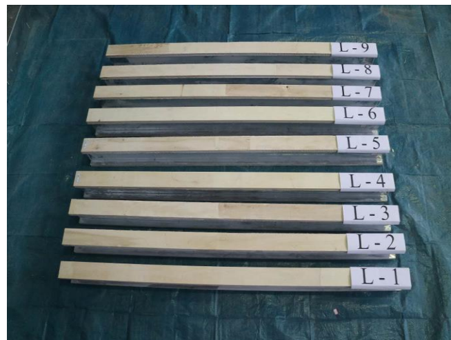
Fig. 2. LVL-steel composite beams
