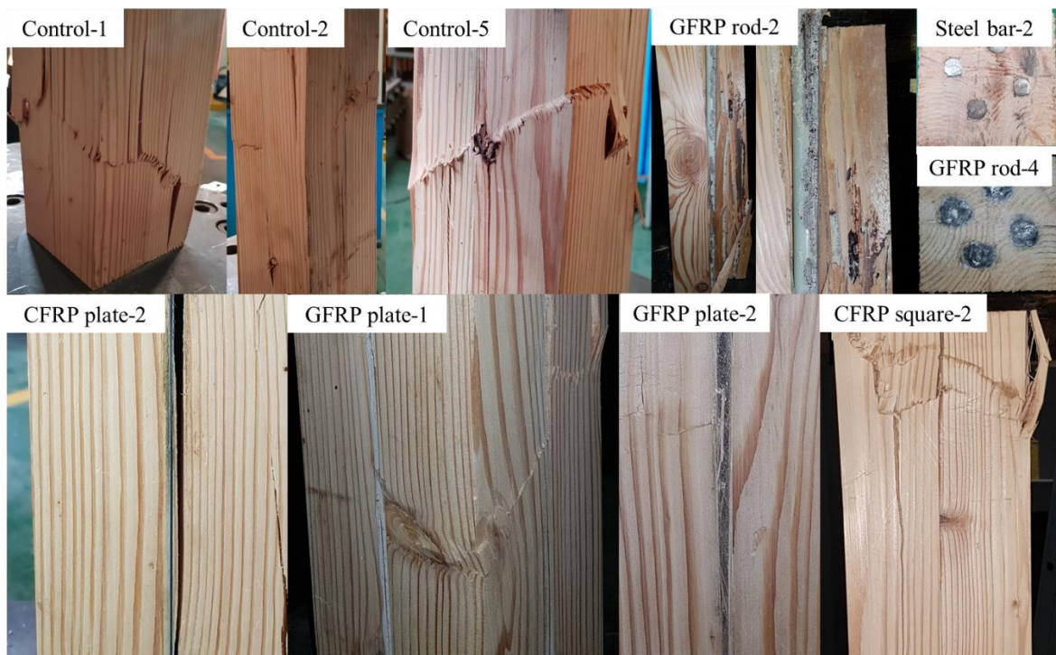
Fig. 4. Photographs of the reinforced-specimen failure modes
