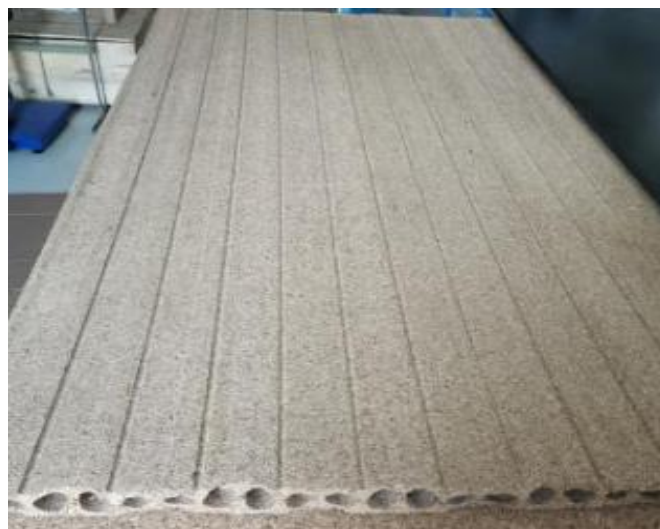
Fig. 6. A 60 mm thick tubular particleboard sample
