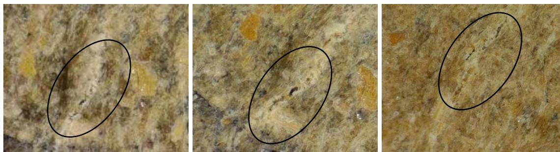
**(a)** G#15 apparent crack (20 d) **(b)** G#15 apparent crack (80 d) **(c)** K#15 apparent crack (80 d)
