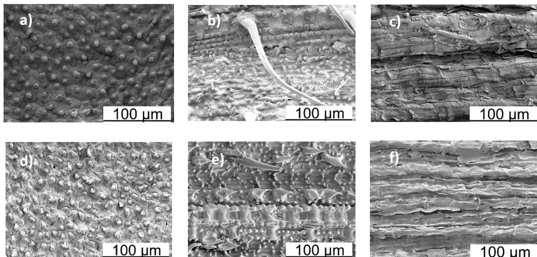
**Fig. 4.** The surface morphology of the untreated a) lotus, b) reed, and c) basho leaves and the treated d) lotus, e) reed, and f) basho leaves
