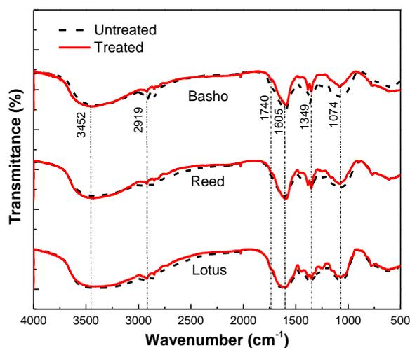
Fig. 1. The FTIR spectra of the treated and untreated leaves
