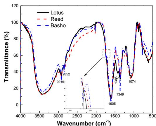
Fig. 2. The FTIR spectra comparison of the treated leaves
