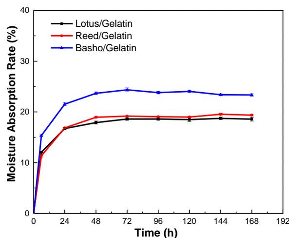
Fig. 7. The moisture absorption curve of the composites
