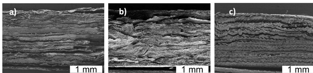
Fig. 5. The cross-section morphology of the a) lotus, b) reed, and c) basho gelatin composites
