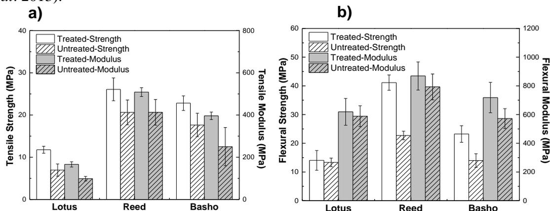
Fig. 6. The a) tensile strength and modulus and the b) flexural strength and modulus of the leaf/gelatin composites
