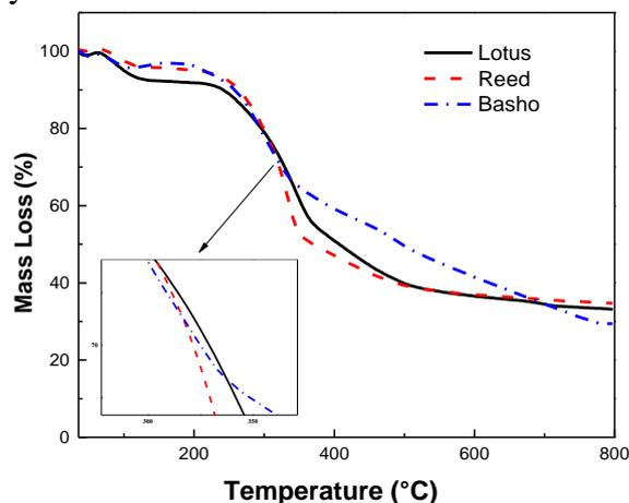
Fig. 3. The TGA curves of the treated leaves
