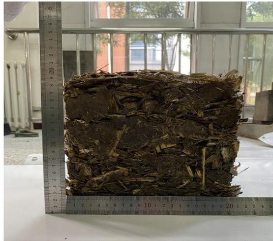
Fig. 5. Compressed briquettes
