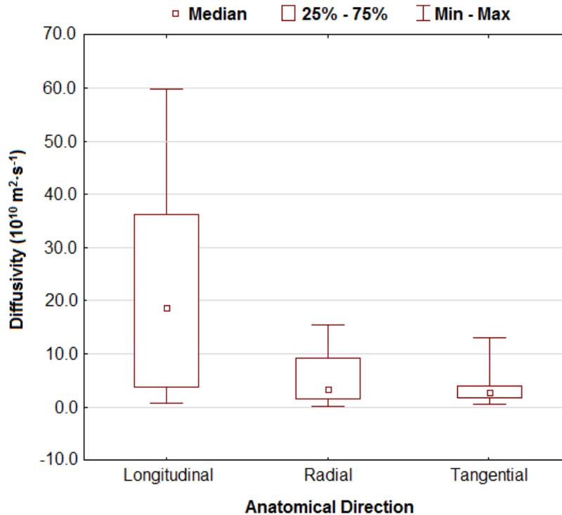
**Fig. 3.** Box-plot graph of diffusion coefficients of the researched degraded wood species; factor anatomical direction
