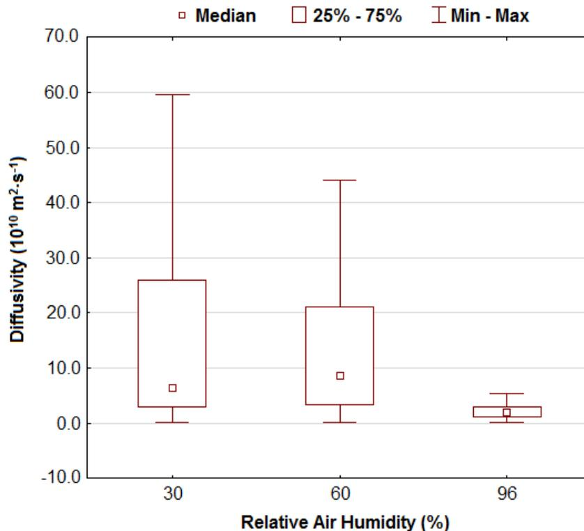
**Fig. 4.** Box-plot graph of diffusion coefficients of the researched degraded wood species; factor relative humidity
