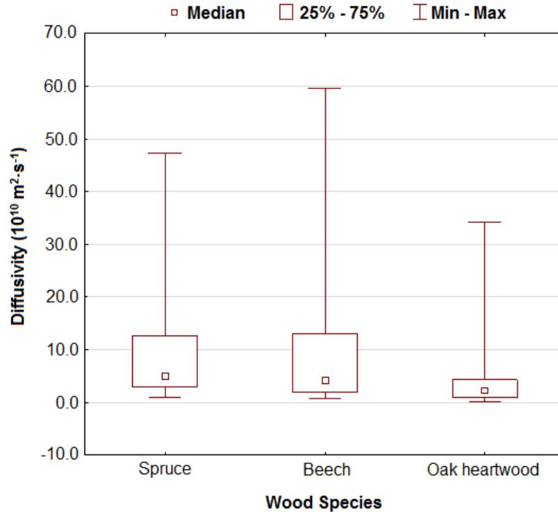
**Fig. 2.** Box-plot graph of the diffusion coefficients of the researched degraded wood species; factor: wood species
