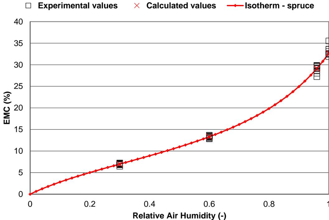
**Fig. 5.** Sorption isotherm of degraded spruce wood
