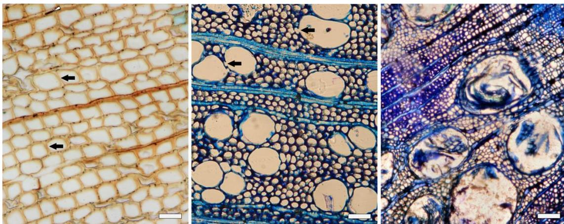
**Fig. 1.** Images of transversal cuts of degraded spruce (on the left), degraded beech (middle) and degraded sessile oak heartwood (on the right). Scale in the images is  $50 \mu\text{m}$  and it is denoted with a light grey stripe at the lower right corner of each image. The black arrows point at visible cell wall thinning and disruptions.
