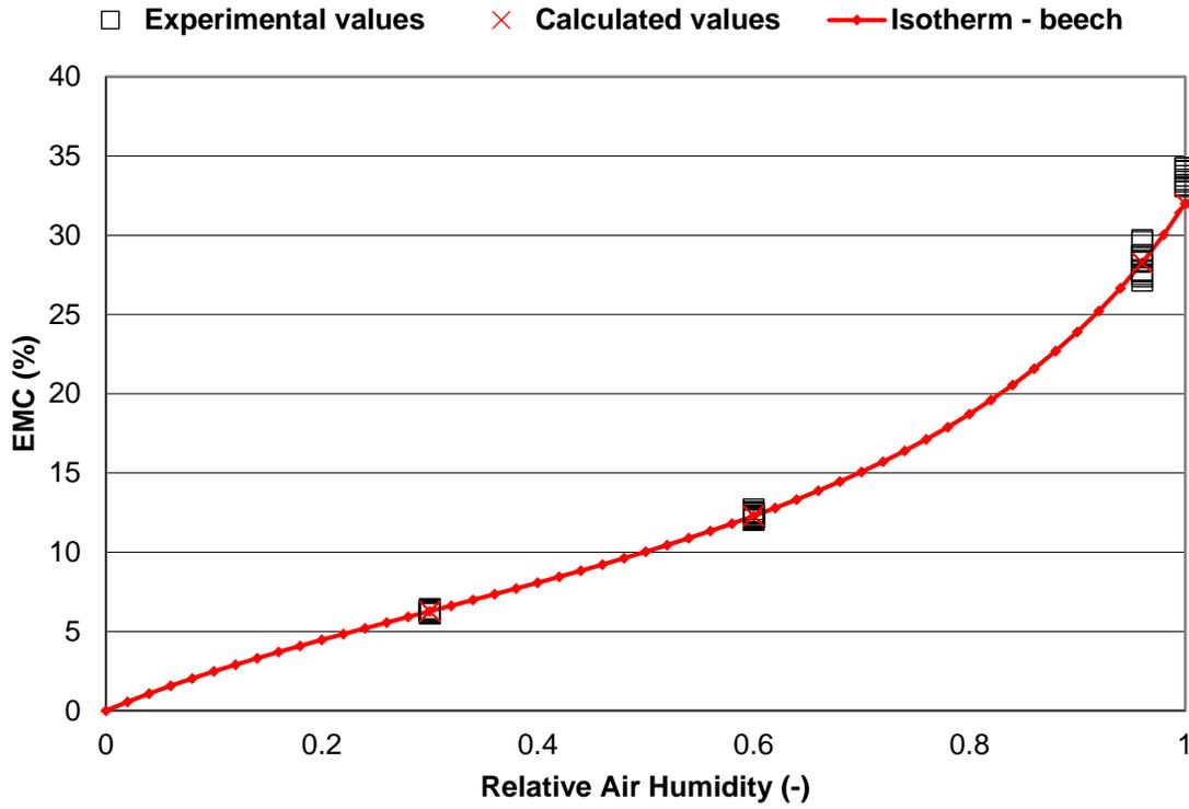
Fig. 6. Sorption isotherm of degraded beech wood
