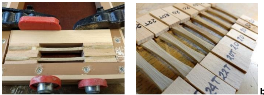
Fig. 3. a) Gluing test samples type dog bone; b) Curing of glued specimens
