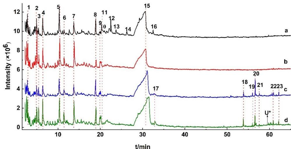
**Fig. 1.** The chromatograms (TIC) obtained *via* Py-GC/MS analysis of (a) bamboo, (b) ramie, (c) mulberry bark, and (d) kozo paper. Note: the peak numbers correspond to the numbers in Table 1
