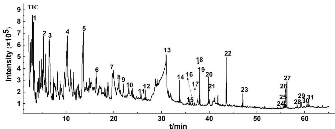
Fig. 4. Total ion current chromatogram obtained from the pyrolysis of Langdu paper
