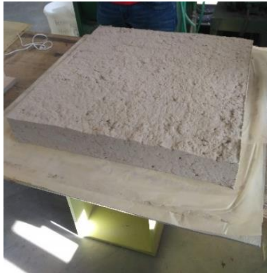
Fig. 2. The pre-formed CB before pressing
