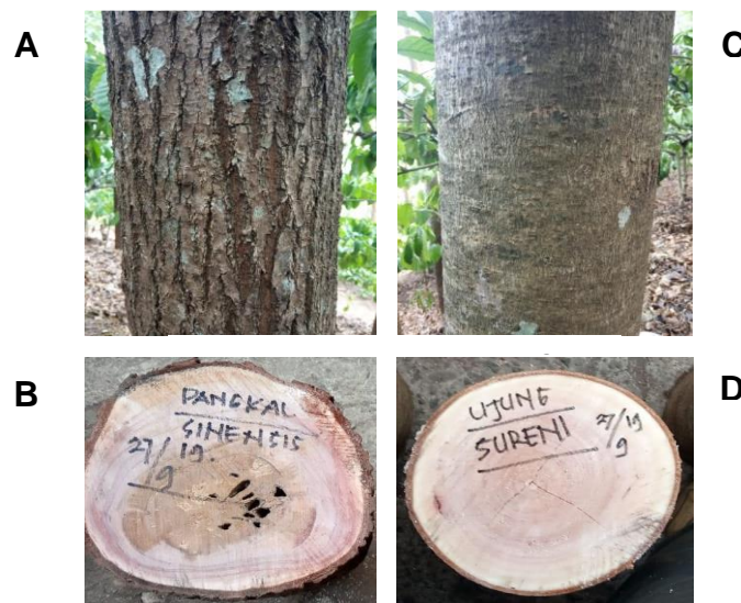
Fig. 2. Gross physical features of both Toona wood species: (A) bark surface of T. sinensis , which is cleaved, rough, and thicker; (B) transversal section of T. sinensis , which is red-brown and darker; (C) bark surface of T. sureni , which is smoother, and thinner; and (D) transversal section of T. sureni , which is white-yellow and brighter
