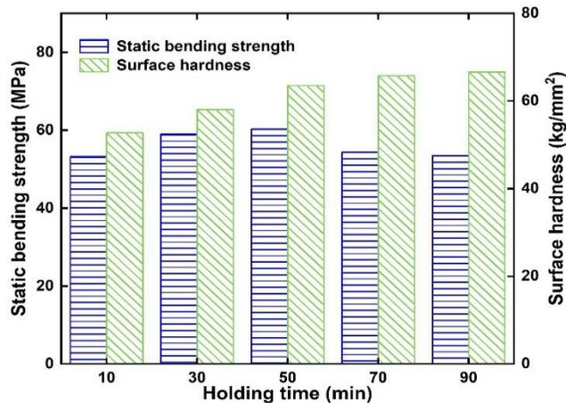
**Fig. 5.** The effect of the holding time on the mechanical properties of compacted wood powder
