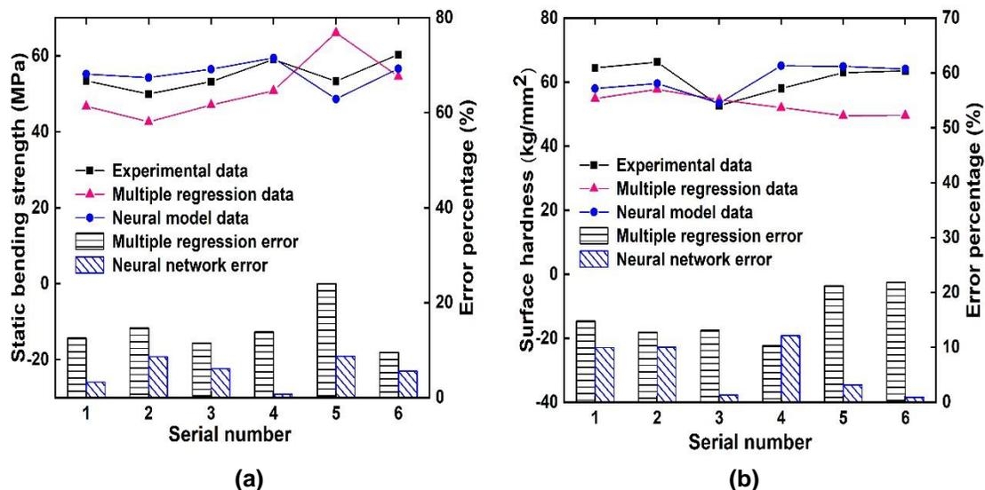
**Fig. 11.** Comparison between the experimental and predicted data of the mechanical properties: (a) static bending strength; and (b) surface hardness
