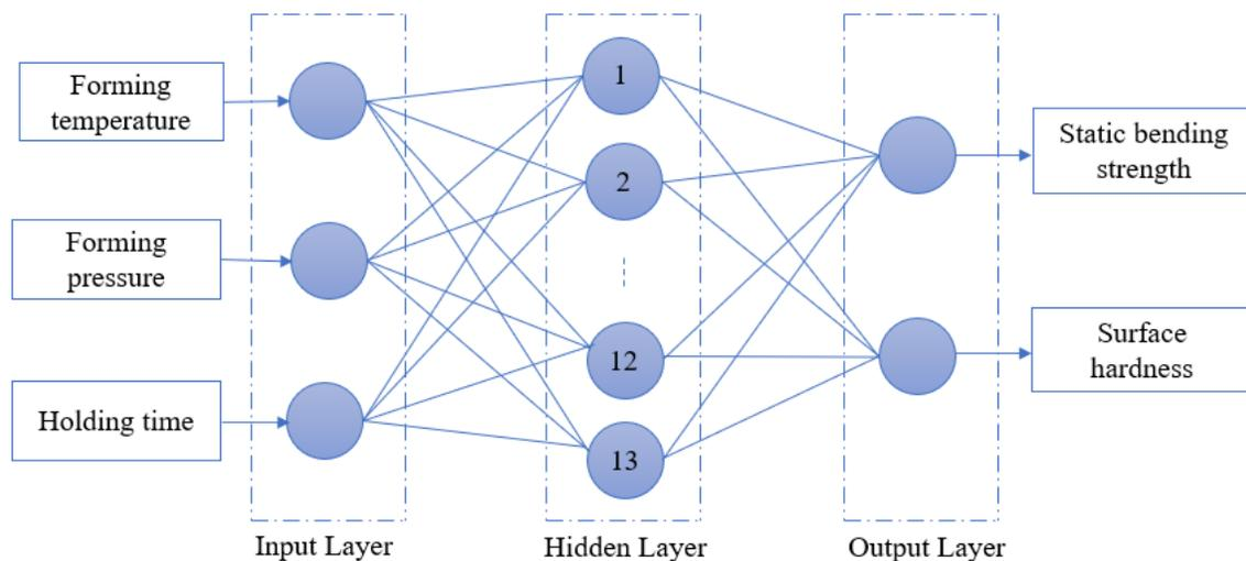
**Fig. 8.** The neural prediction model for the mechanical properties of compacted poplar powder generated via hot-pressing
