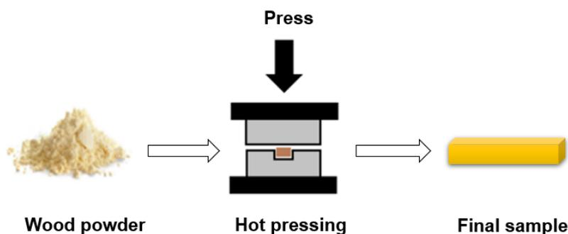
**Fig. 1.** Flow chart of the hot-pressing process
