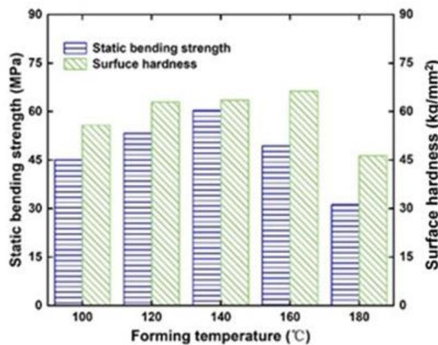
**Fig. 7.** The effect of the forming temperature on the mechanical properties of compacted wood powder
