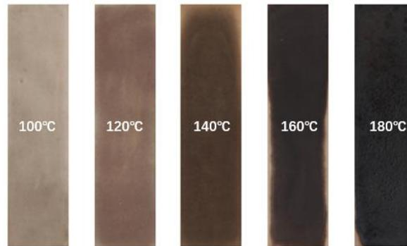
**Fig. 6.** The poplar powder compacts at different forming temperatures
