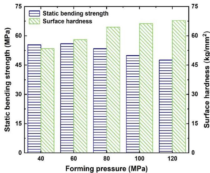
**Fig. 3.** The effect of the forming pressure on the mechanical properties of compacted wood powder
