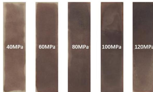
**Fig. 2.** The poplar powder compacts at different forming pressures
