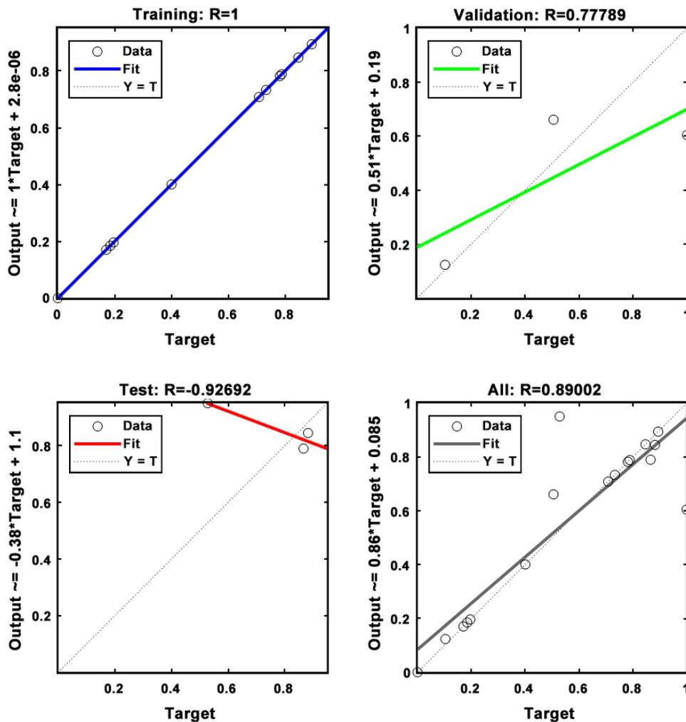
**Fig. 10.** The relationship between the prediction and the experimental data during training, verification, and test of the surface hardness
