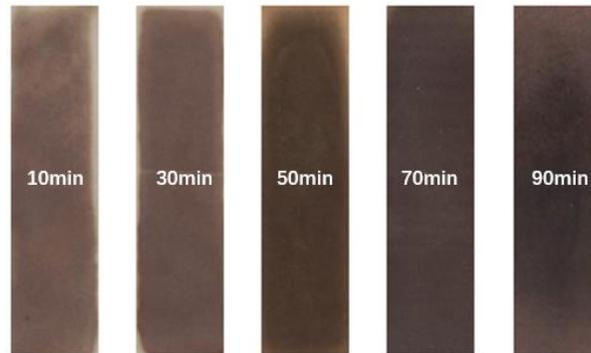
**Fig. 4.** The poplar powder compacts at different holding times
