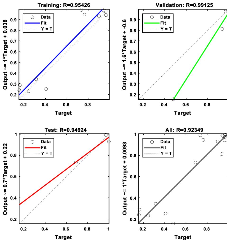
**Fig. 9.** The relationship between the prediction and the experimental data during training, verification, and test of the static bending strength
