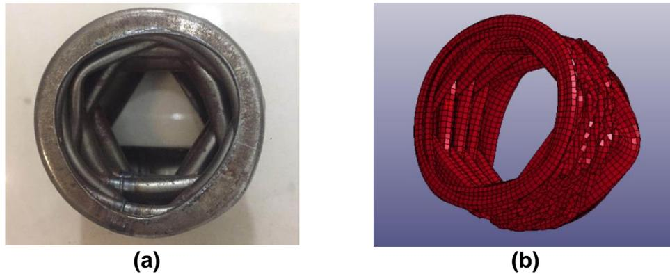
**Fig. 6.** Empty thin-walled tube after crushing test and simulation: (a) Test result; (b) Simulation result
