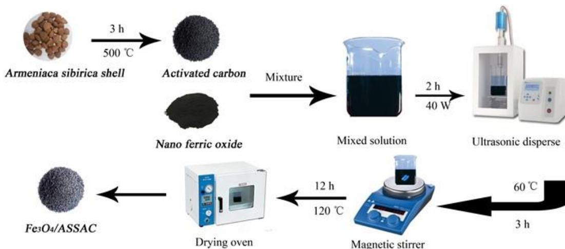
**Fig. 1.** The preparation schematic diagram of  $Fe_3O_4$ /ASSAC
