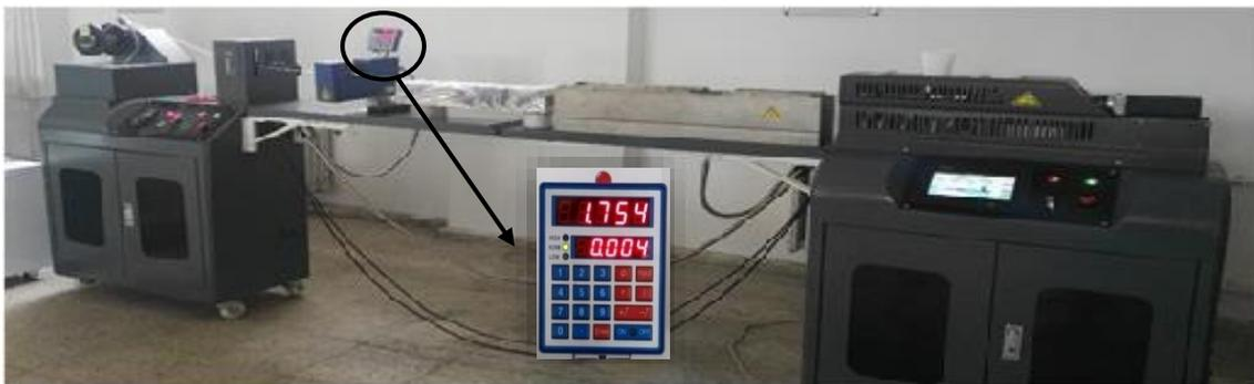
**Fig. 2.** Single screw extruder
