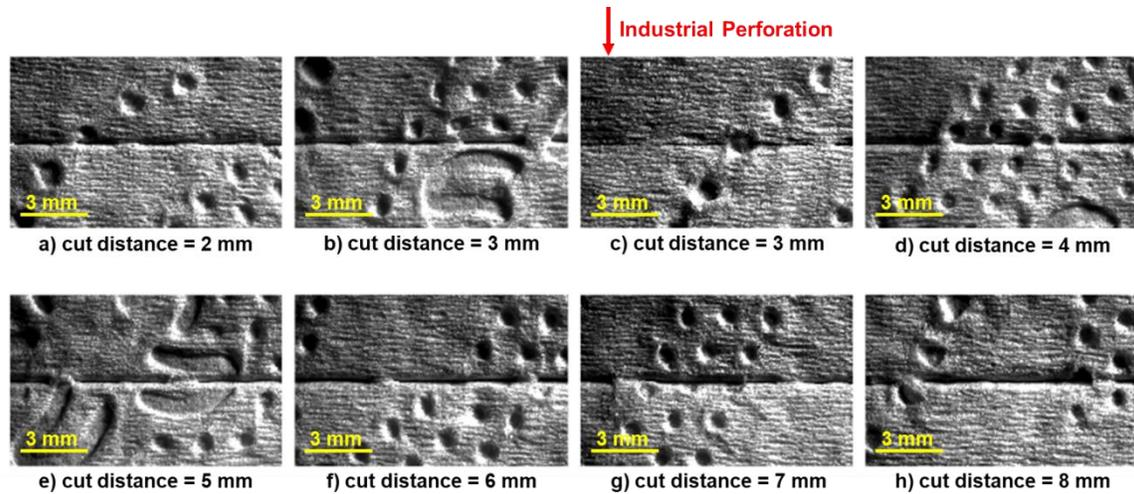
**Fig. 7.** Optical images of the different laboratory cut distances for the BP<sub>2</sub> toilet paper and the industrial perforation for the same toilet paper
