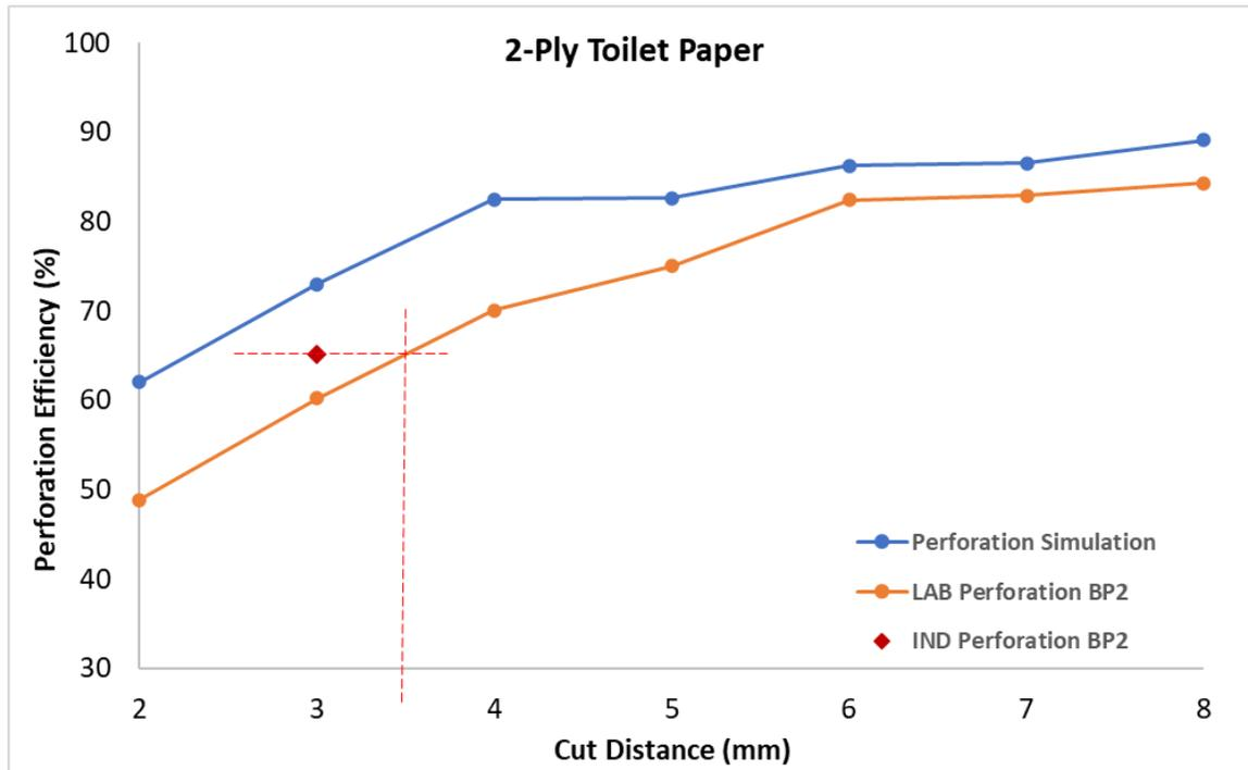
**Fig. 6.** Comparison of the evolution of perforation efficiency with the variation of the cut distances of the FEM simulation, laboratory (LAB) perforation, and industrial (IND) perforation results for a 2-ply toilet paper (BP<sub>2</sub>)
