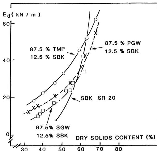
**Fig 13**—Dynamic tensile stiffness of different mechanical pulps at the same freeness level (CSF 90 ml) and a pure chemical pulp as a function of dry solids content.
