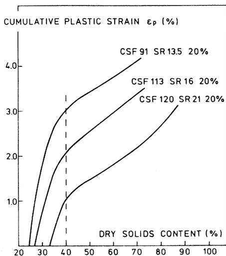
**Fig 16**—Accumulation of plastic strain of TMP/SBK (furnish at different freeness levels during the test (see also Fig 2).
