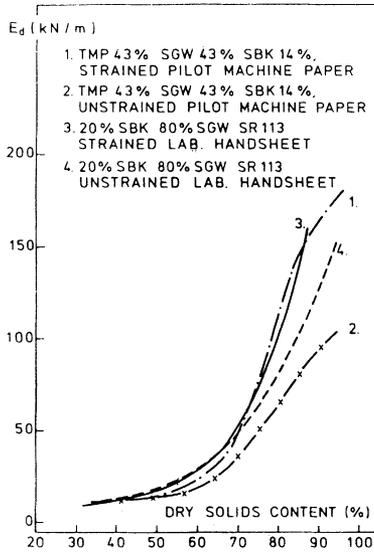
Fig 11—The effect of drying stresses on dynamic tensile stiffness  $E_d$  of different furnishes.
