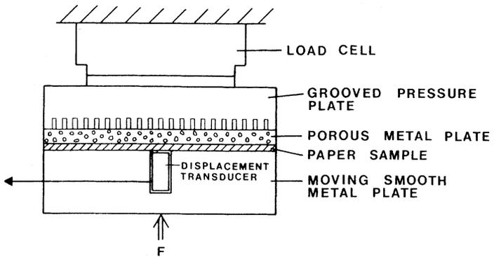
**Fig 3**—The compression plates used in dynamic compressibility measurements.
