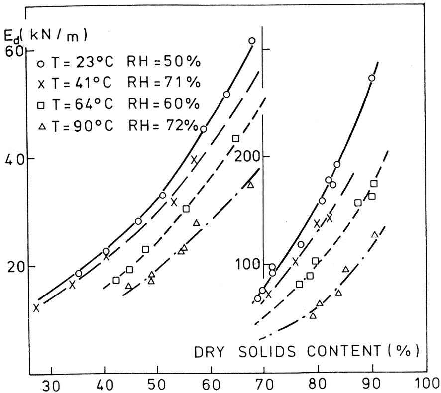
Fig 15—Effect of temperature on the dynamic tensile stiffness of TMP.
