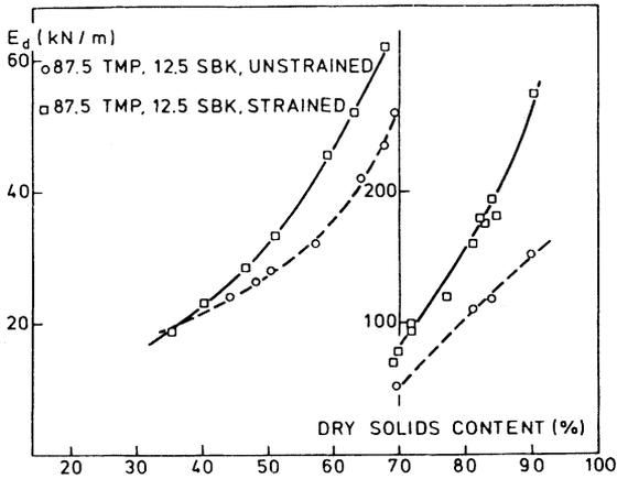
Fig 12—Effect of straining during drying on dynamic tensile stiffness of TMP.
