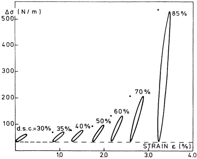
**Fig 2**—Stress-strain behaviour of the sample during dynamic tensile load cycling measurement as a function of increasing dry solids content (d.s.c.).
