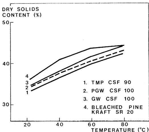
**Fig 18**—Maximum dry solids content of some pulps during wet pressing as a function of temperature.
