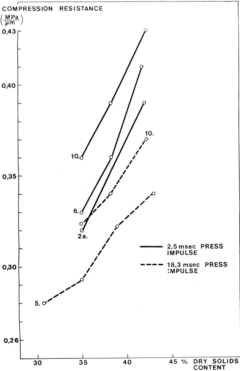
Fig 23—Compression resistance of some pulps as a function of initial dry solids content.
