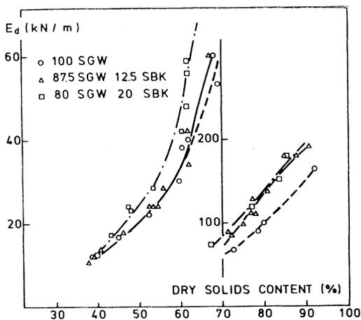
**Fig 14**—Effect of reinforcing chemical pulp (SBK) on dynamic tensile stiffness of newsprint furnish.
