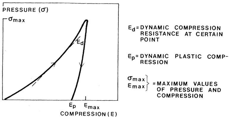
Fig 5—Total pressure in the sample as a function of compression during a dynamic compressibility measurement.
