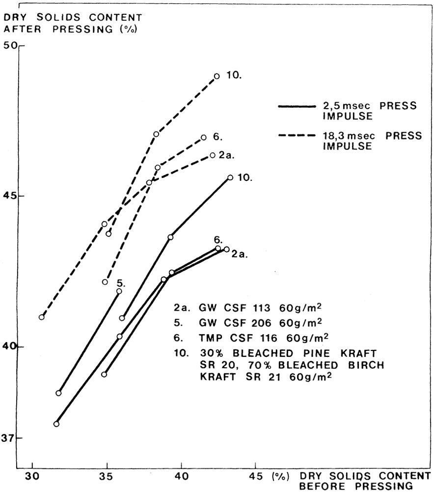
Fig 22—The maximum dry solids content as a function of input dry solids content of some pulps during wet pressing.
