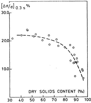
**Fig 6**—Relative tensile stress (relaxation  $(\Delta\sigma/\sigma)$ , 3 sec (%)) (percentage relaxation of stress in 300 m sec) of a newsprint furnish as a function of dry solids content.
