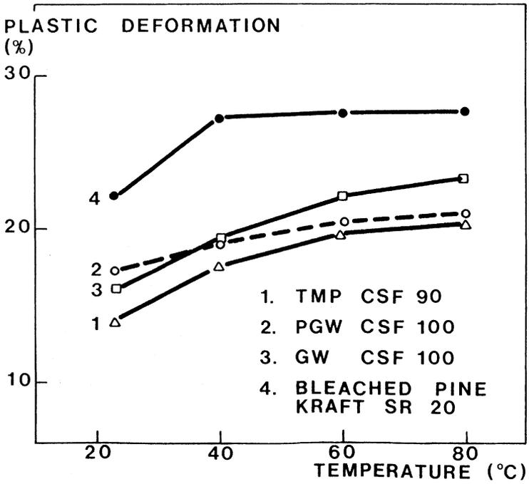
**Fig 19**—Relative plastic deformation of different pulps in z-direction as a function of temperature based on 2.2 m sec press impulse of 4.5 MPa.
