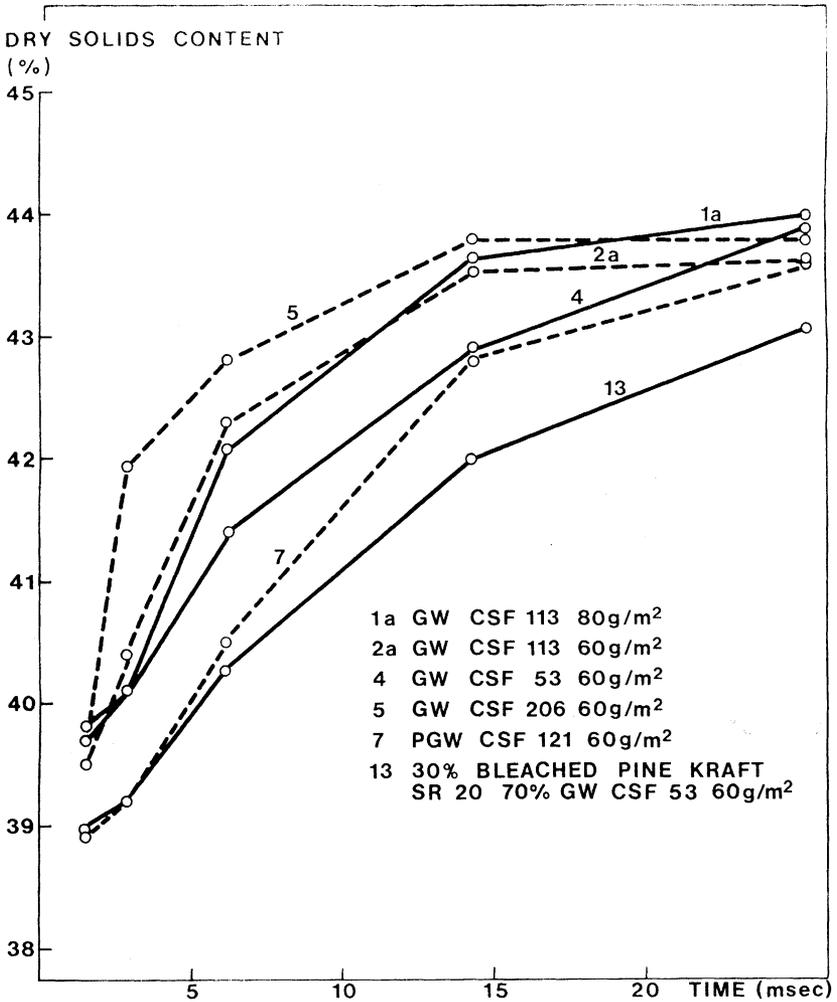
Fig 21—Effect of press impulse duration on the maximum dry solids content of different pulps.
