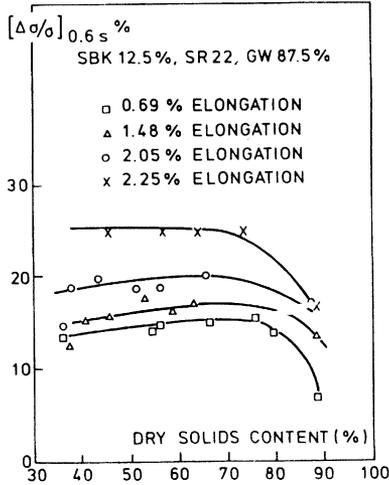
Fig 10—Relative tensile stress relaxation (percentage relaxation of stress in 600 m sec) of a newsprint furnish at different strain levels.
