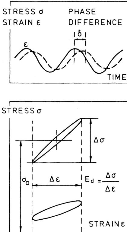
Fig 1—Principle of the dynamic elasticity and visco-elasticity measurement in time-base and in a stress-strain diagram.
