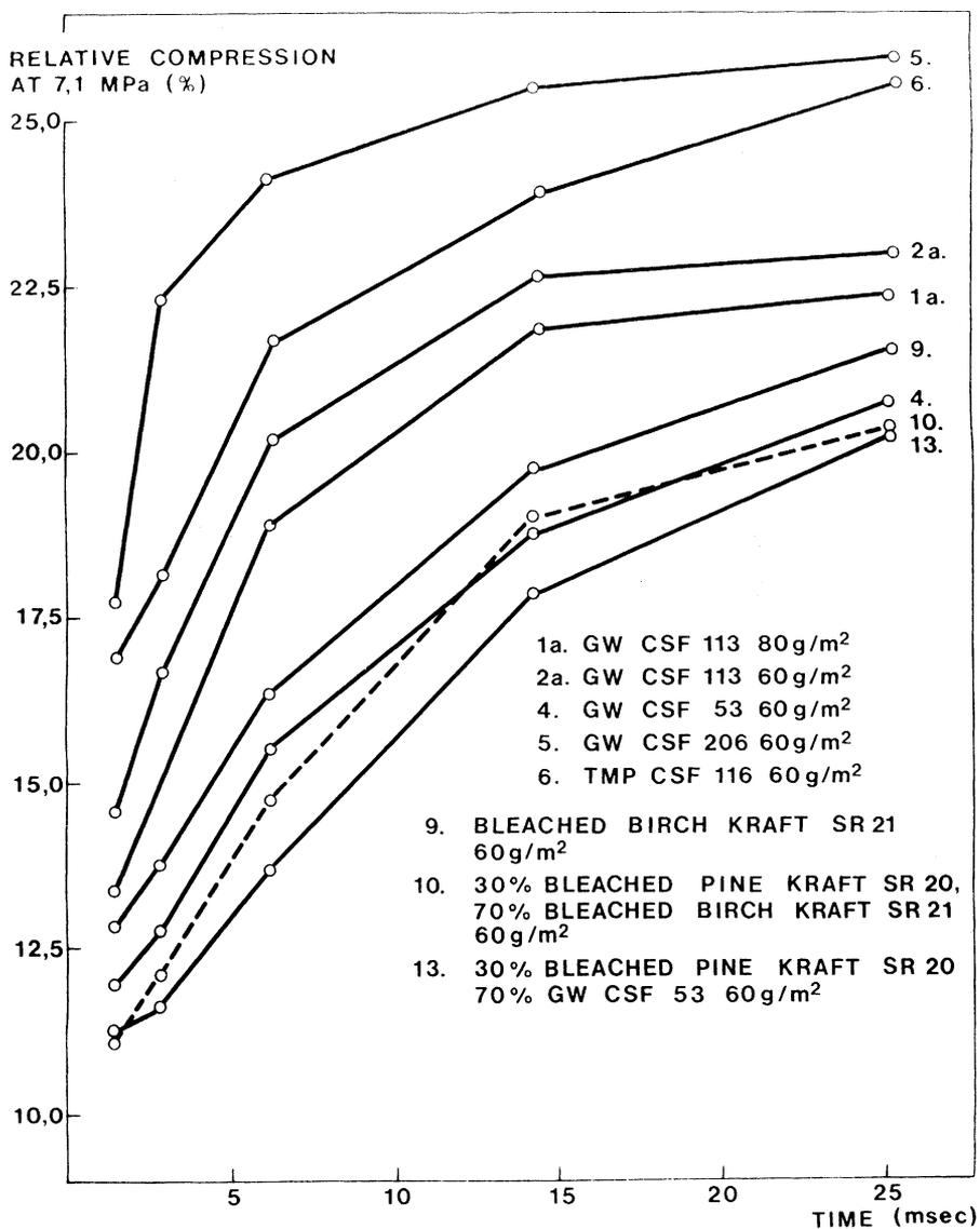
Fig 20—The relative compression of different pulps as a function of press impulse duration.
