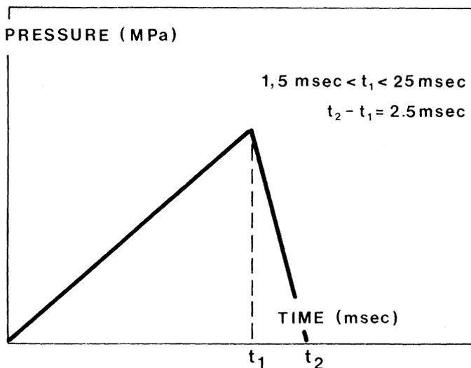
Fig 4—The pressure impulses used in dynamic compressibility measurements.
