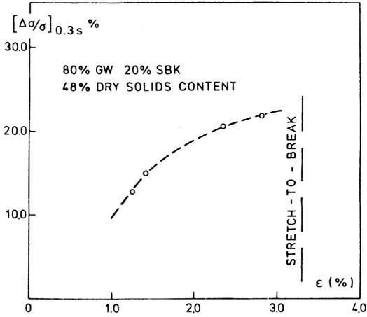
Fig 9—Effect of strain on relative tensile stress relaxation.
