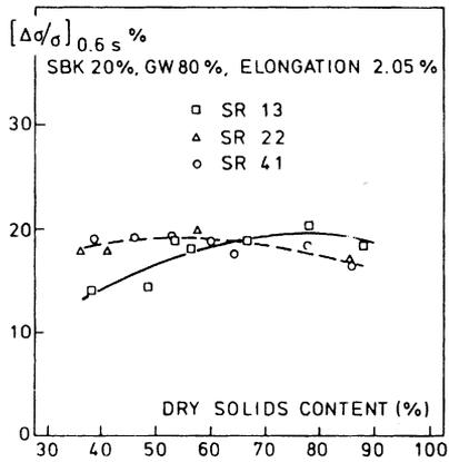
**Fig 8**—Effect of beating of the reinforcing pulp on relative tensile stress relaxation in a newsprint furnish.
