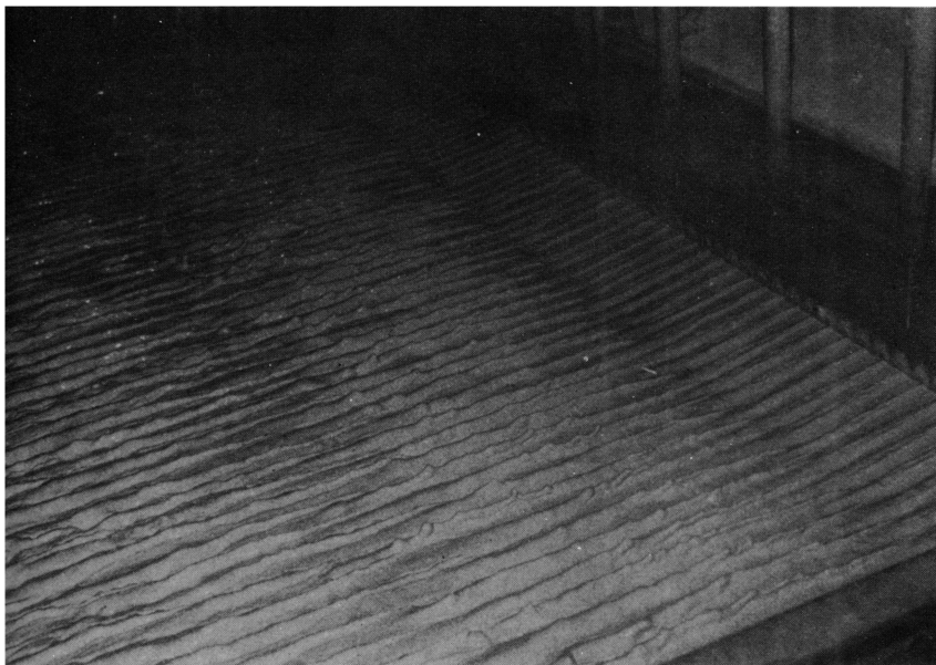
Fig 21 —Ridges of a serrated slice travelling at 700 m/min
