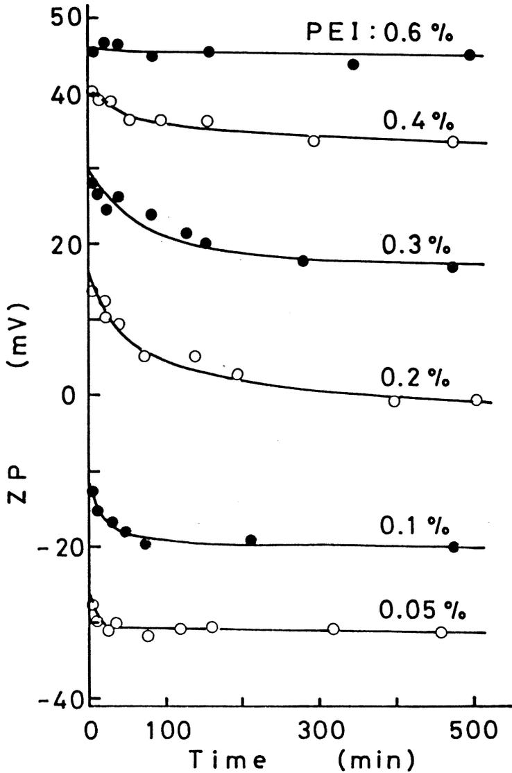
**Fig 16**—Change in zeta potential of PEI-treated clay at various addition levels with agitation of 750 rpm. (Conditions are the same as those in Fig.11 except MW of PEI) MW of PEI; 1,800
