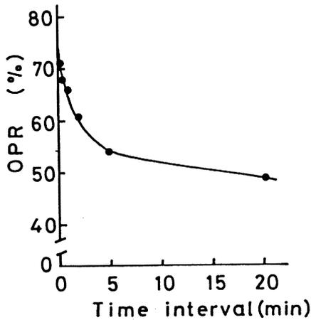
**Fig 24**—Effect of time interval between the additions of PEI and A-PAM on OPR of fines in dual polymer system. PEI; 0.05 % on solid (added first). A-PAM; 0.05 % on solid (after certain min), Agitation; 1,000 rpm
