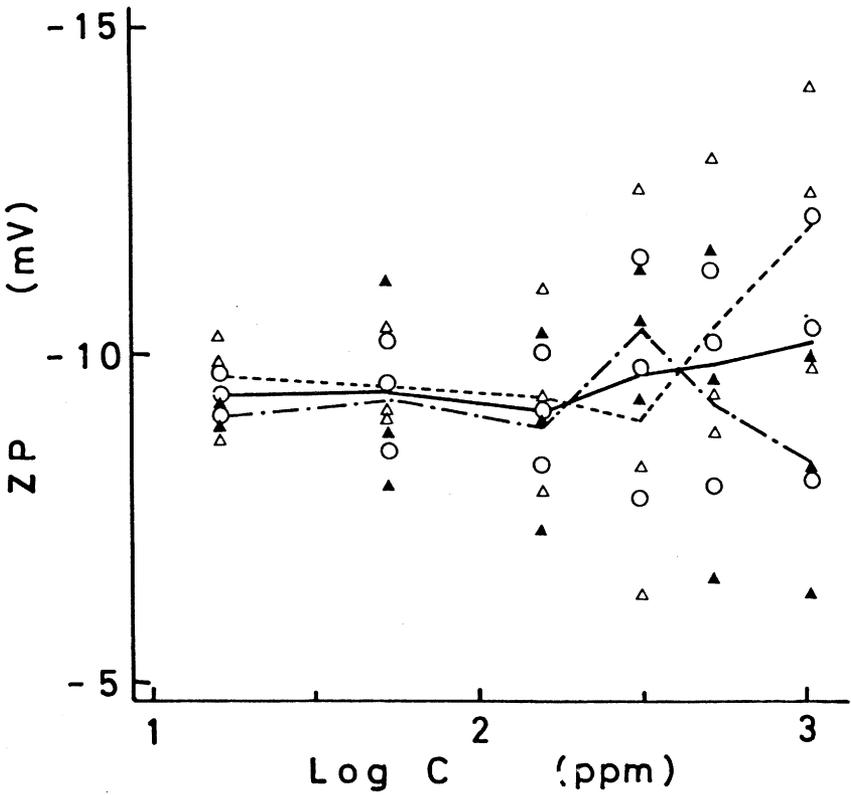
**Fig 10**—The zeta potential of pulp fines measured at a concentration (C) of 15 to 1050 ppm in a lateral arrangement of a flat cell. (20-23°C, pH 7.5, 0.32 mS/cm, 0.35 mA)
