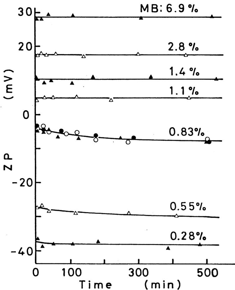
**Fig 13**—Change in zeta potential of MB-treated clay at various addition levels under various turbulences. (18-21°C, pH 5.7, 0.50 mS/cm, 0.60 mA, NaCl 0.0045 M)
