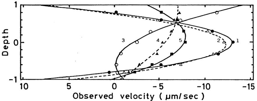
**Fig 1**—Velocity distribution curve of kaolin particles at a horizontal arrangement of a conventional cell or cell pretreated with PEI. ( $20 \pm 1^\circ\text{C}$ , pH 7.4,  $0.27 \text{ mS/cm}$ ,  $0.25 \text{ mA}$ ) No.1 and No.2; conventional cell, about 5% (No.1) or 50% (No.2) of the bottom surface area was covered with kaolin particles after measurements while the top surface area was little covered.
