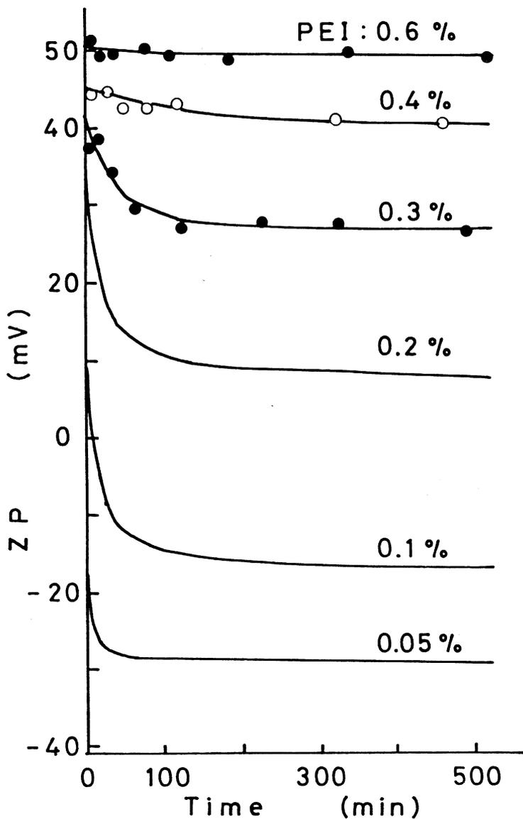
**Fig 11**—Change in zeta potential of PEI-treated clay at various addition levels with agitation of 750 rpm. (18-21°C, pH 6.0, 0.50 mS/cm, 0.60 mA, NaCl 0.0045 M) Clay; 300 ppm, Molecular weight (MW) of PEI; 80,000
