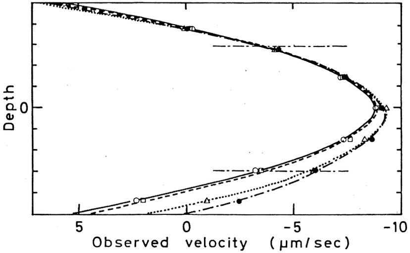
**Fig 6**—Velocity distribution curve of clay particles in various concentrations at a horizontal arrangement of a flat cell. (20-22°C, pH 7.8, 0.32 mS/cm, 0.20 mA)
