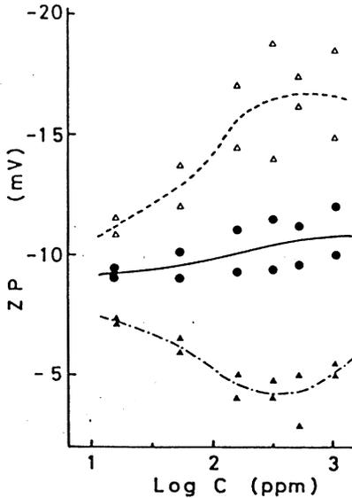
Fig 7—The zeta potential of pulp fines measured at a concentration (C) of 15 to 1050 ppm in a horizontal arrangement of a flat cell with 3.92 mm height. (20-23°C, pH 7.5, 0.32 mS/cm, 0.35 mA)
