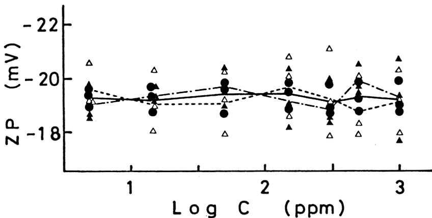
**Fig 9**—The zeta potentation of clay particles measured in the concentration (C) of 5 to 1000 ppm at a lateral arrangement of a flat cell. (20-22°C, pH 7.8, 0.32 mS/cm, 0.35 mA)
