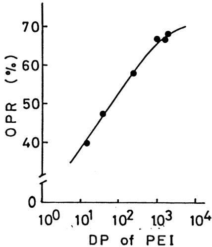
**Fig 23**—Effect of DP of PEI on OPR of fines in dual polymer system. PEI; 0.05 % on solid (added first), A-PAM; 0.05 % on solid (after 0.5 min), Agitation; 1,000 rpm
