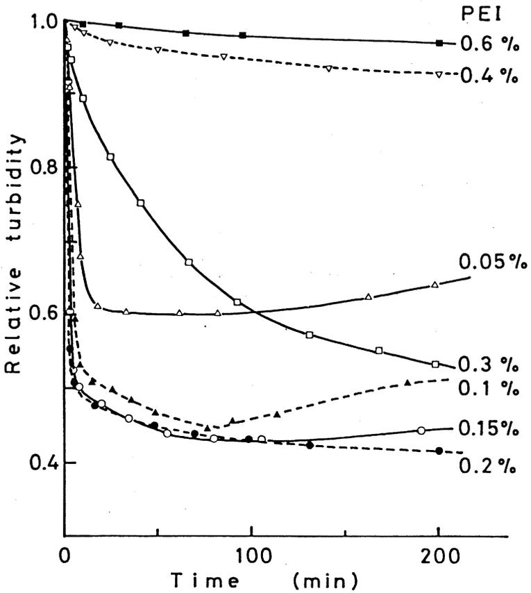
**Fig 21**—Effects of PEI dosage and agitation on flocculation of PSL. (18-20°C, pH 6.0, NaCl 0.0045 M) PSL; 60 ppm, 750 rpm
