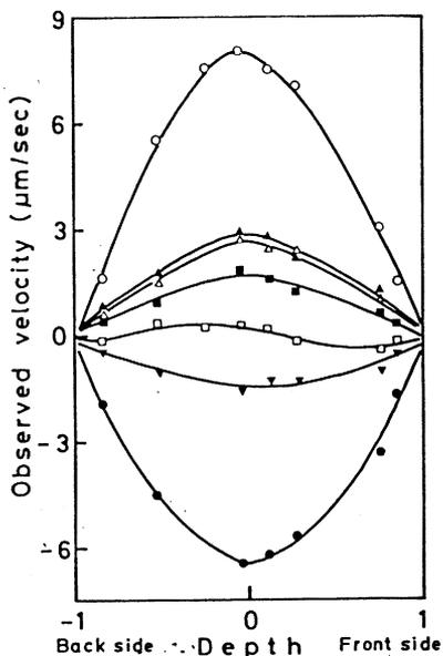
**Fig 8**—The falling or rising velocity of clay particles at a lateral arrangement of a flat cell under the microscope illumination shaded by water in the glass cell with a base 5x2 cm and a height of 5 cm. Degree of shade under a full scale(10.0) illumination(%);
