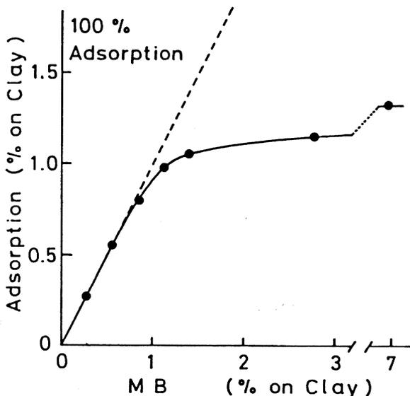
Fig 14—Adsorption of MB onto clay. (20°C, pH 5.7, NaCl 0.0045 M)
