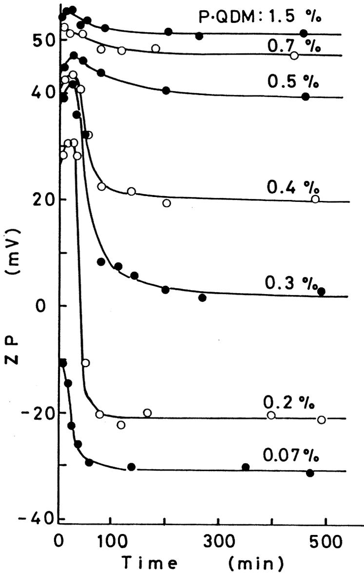
Fig 19—Change in zeta potential of P-QDM-treated clay at various addition levels with agitation of 750 rpm. (18-21°C, pH 5.8, 0.50 mS/cm, 0.60 mA, NaCl 0.0045 M) Clay; 300 ppm
