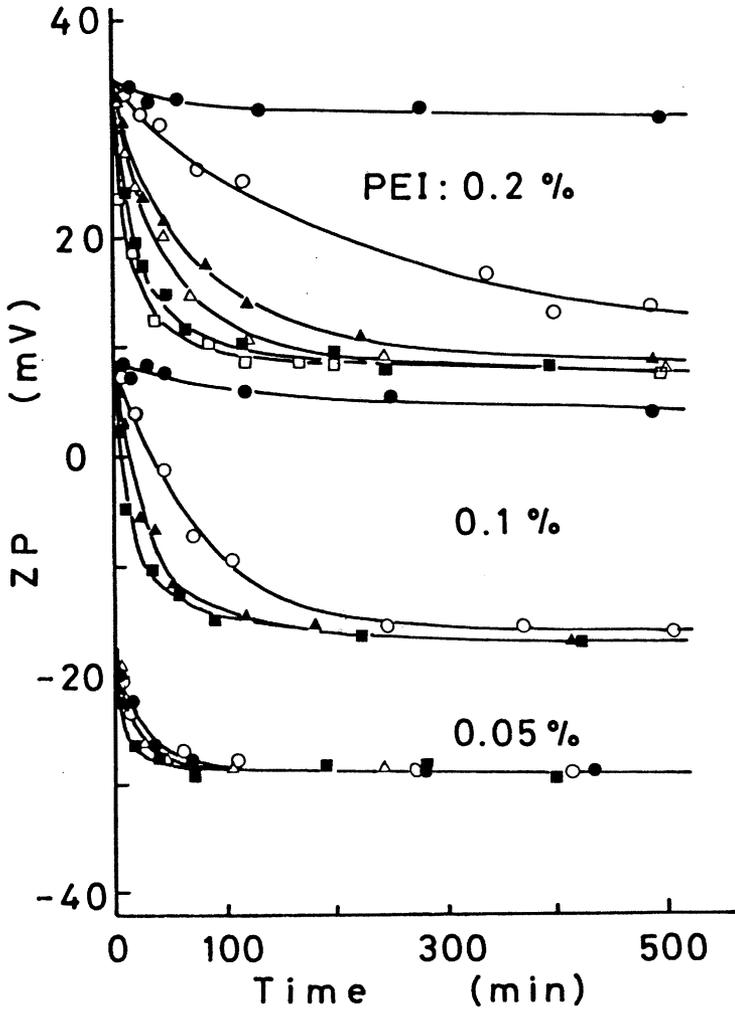
**Fig 12**—Change in zeta potential of PEI-treated clay at various addition levels under various turbulences. (Conditions are the same as those in Fig.11)
