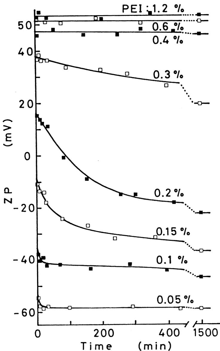
Fig 15—Change in zeta potential of PEI-treated PSL at various addition levels with agitation of 750 rpm. (18-21°C, pH 6.0, 0.50 mS/cm, 0.60 mA)
