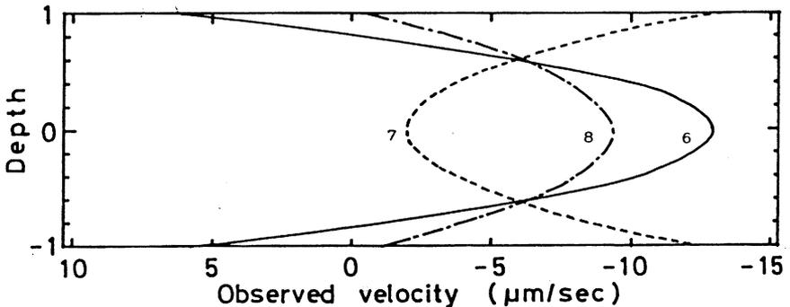
**Fig 2**—Velocity distribution curve of fine pulps at a horizontal arrangement of a conventional cell or cell pretreated with PEI. ( $20 \pm 1^\circ\text{C}$ , pH 7.5,  $0.27 \text{ mS/cm}$ ,  $0.25 \text{ mA}$ )
