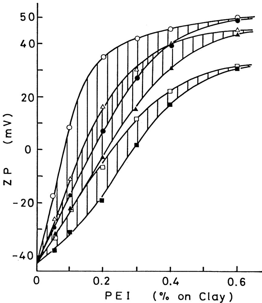
**Fig 18**—Difference in zeta potential of PEI-treated clay between initial and equilibrium stages at various addition levels. (Conditions are shown in Figs 11, 16 and 17)
