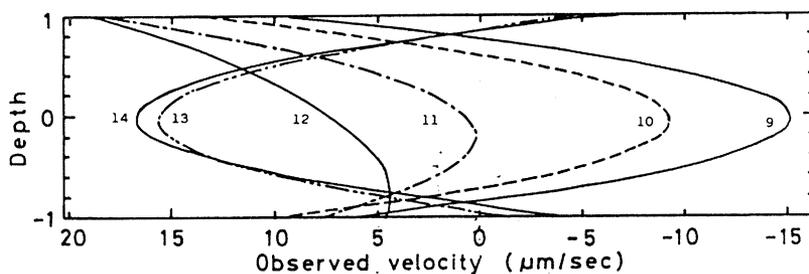
**Fig 3**—Effect of PEI on distributions of migration velocities and Up of kaolin particles at a horizontal arrangement of a flat cell.
