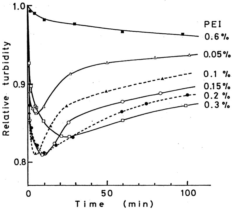
Fig 20—Effects of PEI dosage and agitation on flocculation of clay. (18-20°C, pH 6.0, NaCl 0.0045 M) Clay; 300 ppm, 750 rpm
