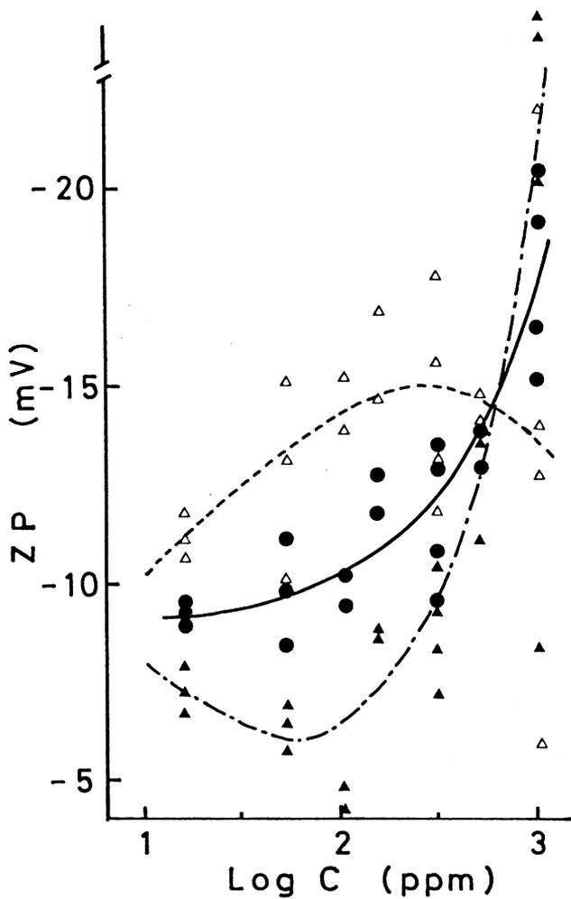
**Fig 5**—The zeta potential of pulp fines measured in the concentration (C) of 15 to 1050 ppm at a horizontal arrangement of a flat cell (23-25°C, pH 7.5, 0.32 mS/cm, 0.35 mA)
