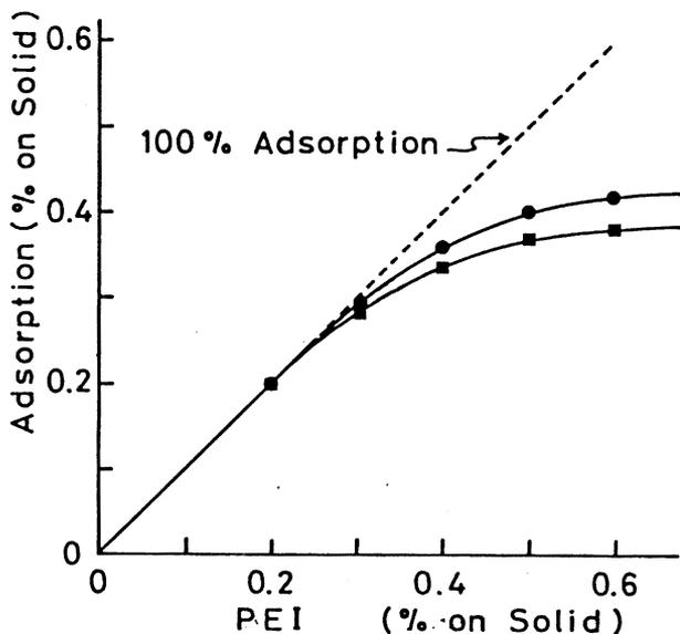
**Fig 22**—Adsorption of PEI onto clay and PSL. (20°C, pH 6.0, NaCl 0.0045 M) MW of PEI; 80,000, ● ;Clay, ■ ;PSL
