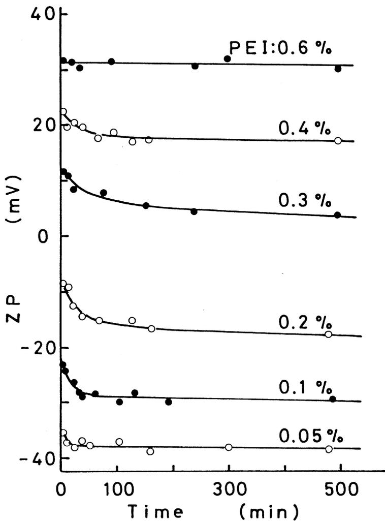
Fig 17—Change in zeta potential of linear PEI-treated clay at various addition levels with agitation of 750 rpm. (Conditions are the same as those in Fig 11 except characters of PEI) MW of linear PEI; 1,700
