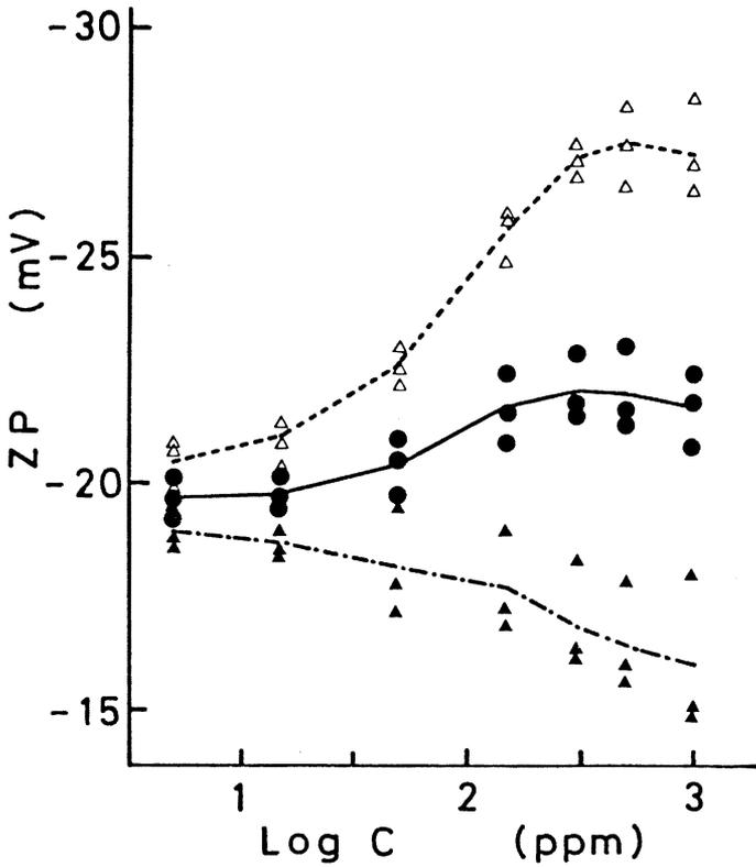
**Fig 4**—The zeta potential of clay particles measured in the concentration (C) of 5 to 1000 ppm at a horizontal arrangement of a flat cell.
