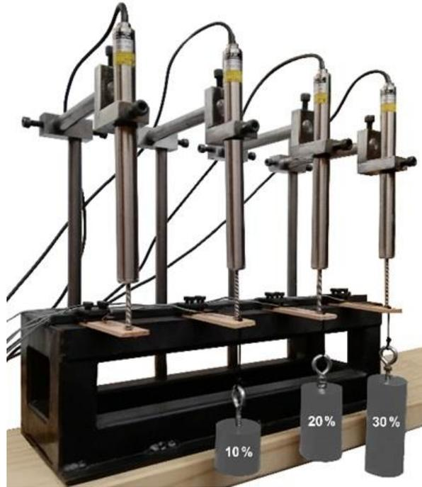
**Fig. 2.** Assembly of the test: four beams installed in cantilever exposed to different conditions of concentrated load (no load, 10%, 20%, and 30%), with continuous monitoring of stresses and vertical displacement
