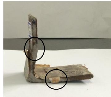
(b) Bending deformation of connector
