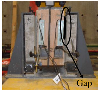
(a) Gap between timber and concrete
