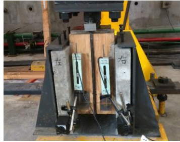
(a) Test apparatus and displacement gauge
