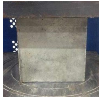
(b) Compressive test of concrete cubes
