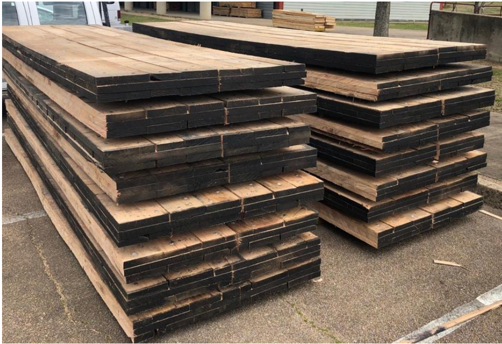
Fig. 2. Stack of three-ply solid mat flexural specimens cut and prepared for testing
