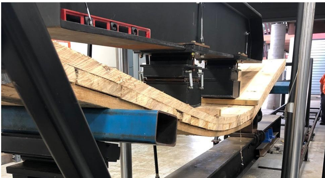
Fig. 4. Three-ply solid flexural specimen in the universal testing machine while being destructively evaluated
