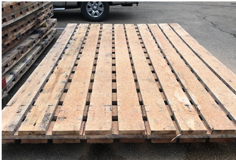
Fig. 3. Three-ply waffle parent mat after ripping into four, 2-foot wide, flexural test specimens
