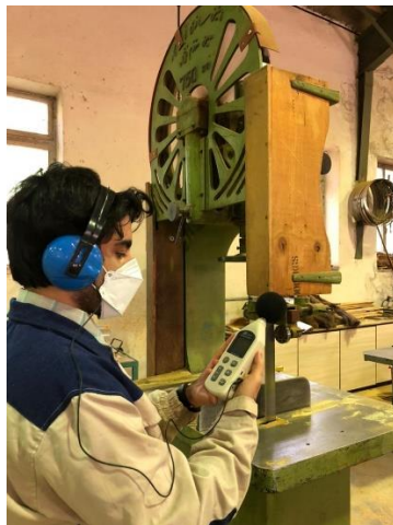
Fig. 2. Positioning of the operator in the evaluation of sound emission in the band saw
