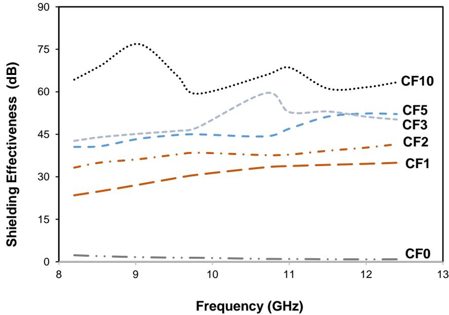
Fig. 3.  $SE_T$  of the MDF panels with different CF addition levels
