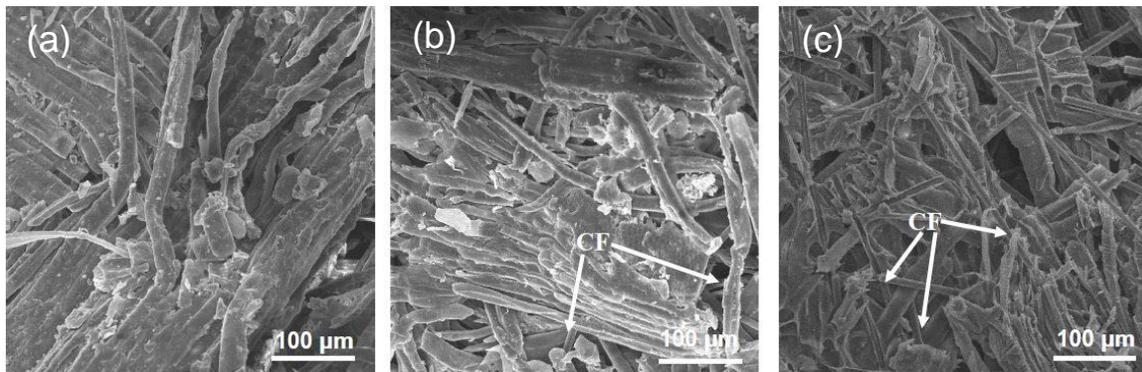
**Fig. 2.** The FE-SEM images (at 500X magnifications) from the surface of the MDF (a. CF0, b. CF10, and c. CF10)
