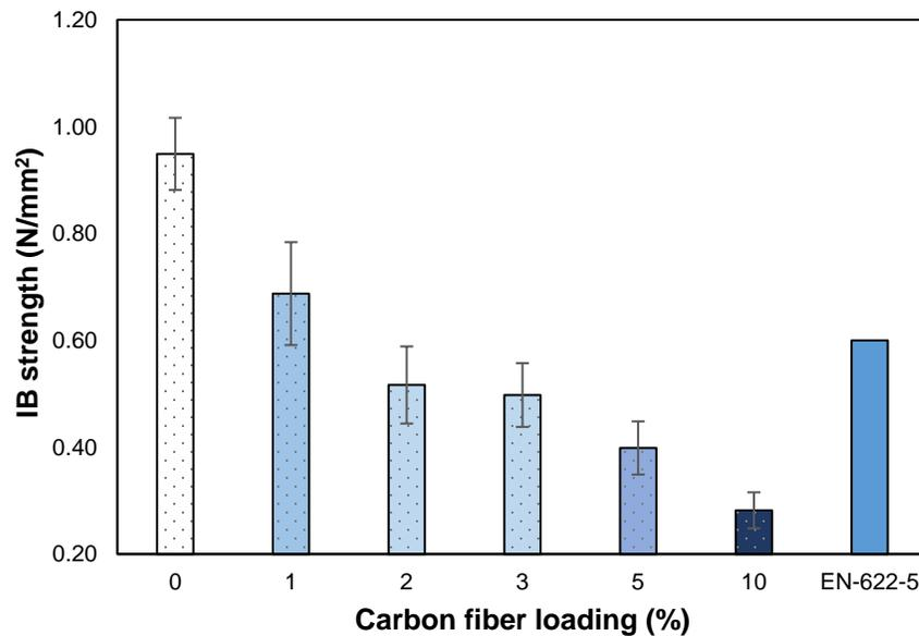
Fig. 5. The IB strength of the MDF panels with different CF loading rates
