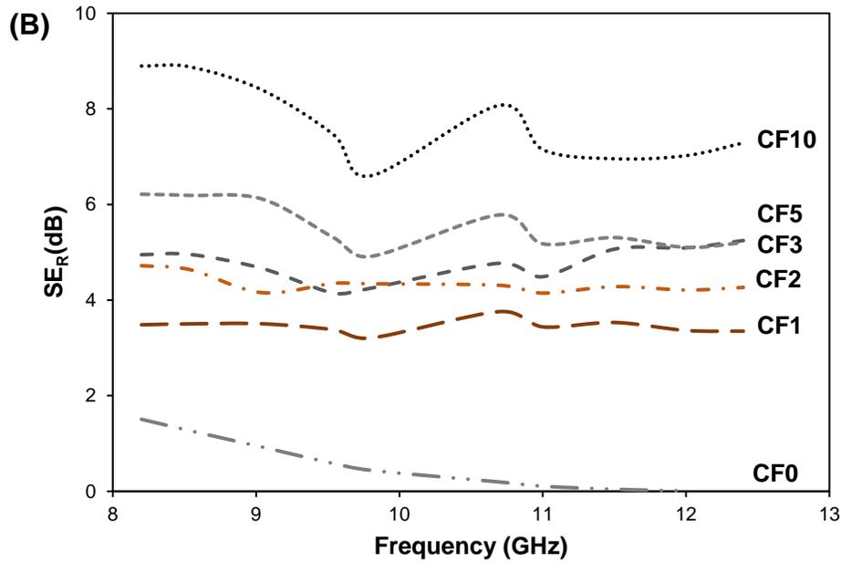
Fig. 4. The (A)  $SE_A$  and (B)  $SE_R$  values of the MDF panels with different CF addition levels.
