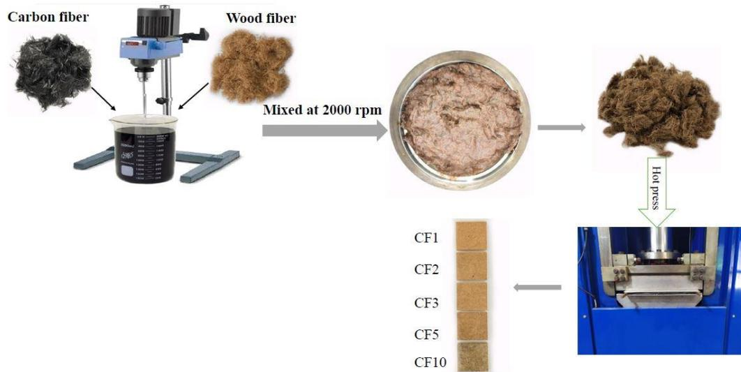
**Fig. 1.** Schematic for the production process CF-filled fiberboard
