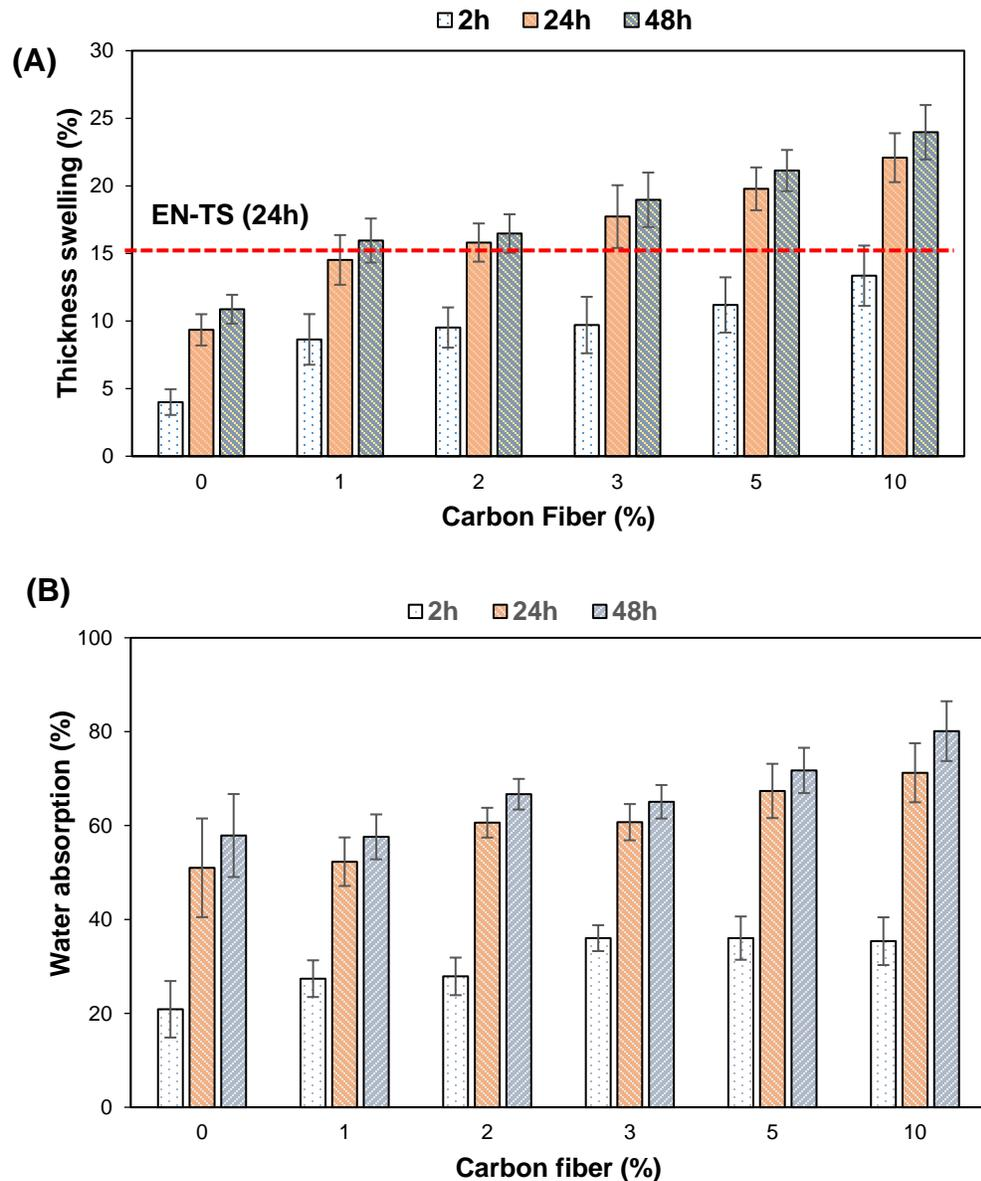
Fig. 7. The (A) TS and (B) WA properties for the MDF panels with different CF addition rates.
