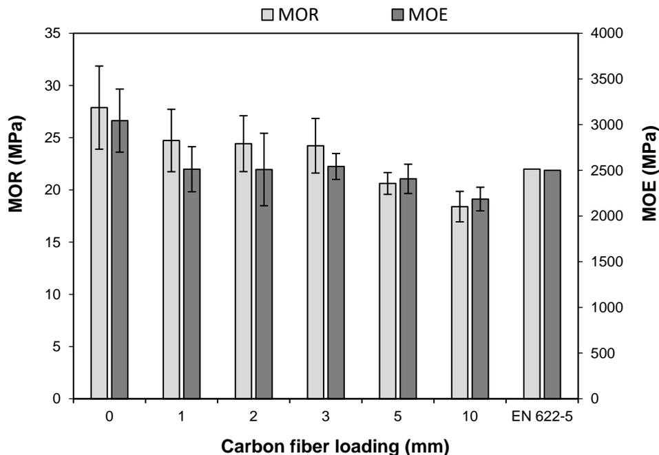
Fig. 6. MOR and MOE values for the MDF panels with different CF addition rates
