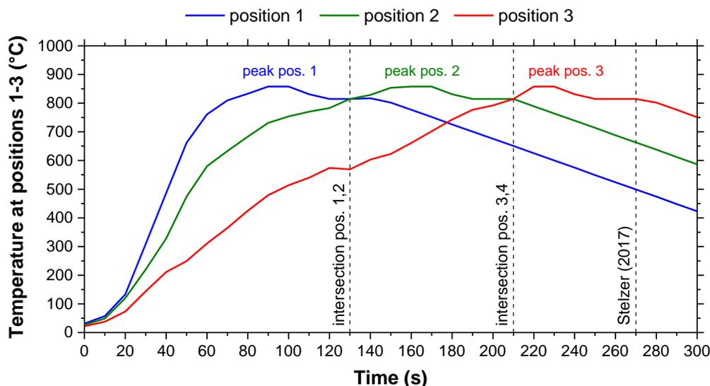
Fig. 4. Hypothesized temperature-time diagram for the three optimal temperature curves
