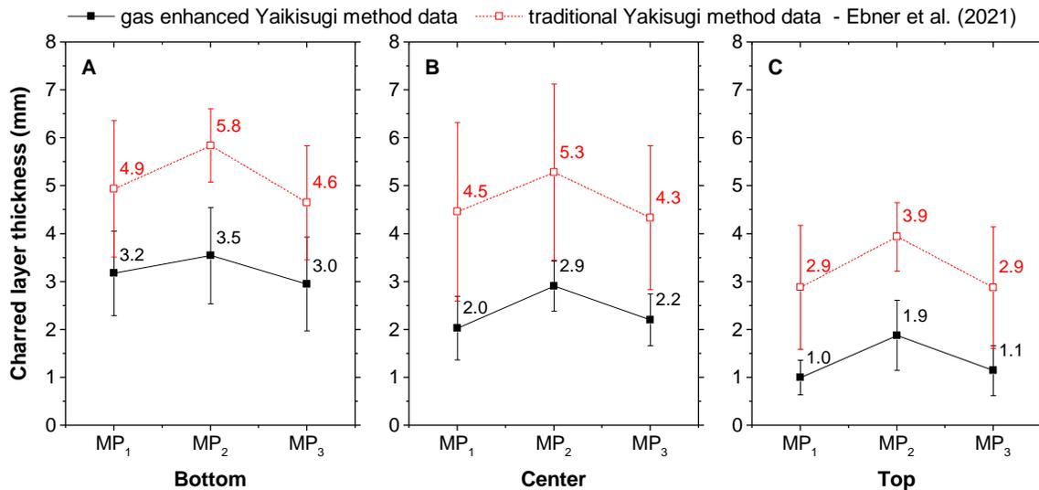
**Fig. 5.** The charred layer thickness at: cut line 1 – bottom (A); cut line 2 – middle (B); and cut line 3 - top (C) compared with previously measured data by Ebner *et al.* (2021) (Note: the error bars represent the standard deviation)
