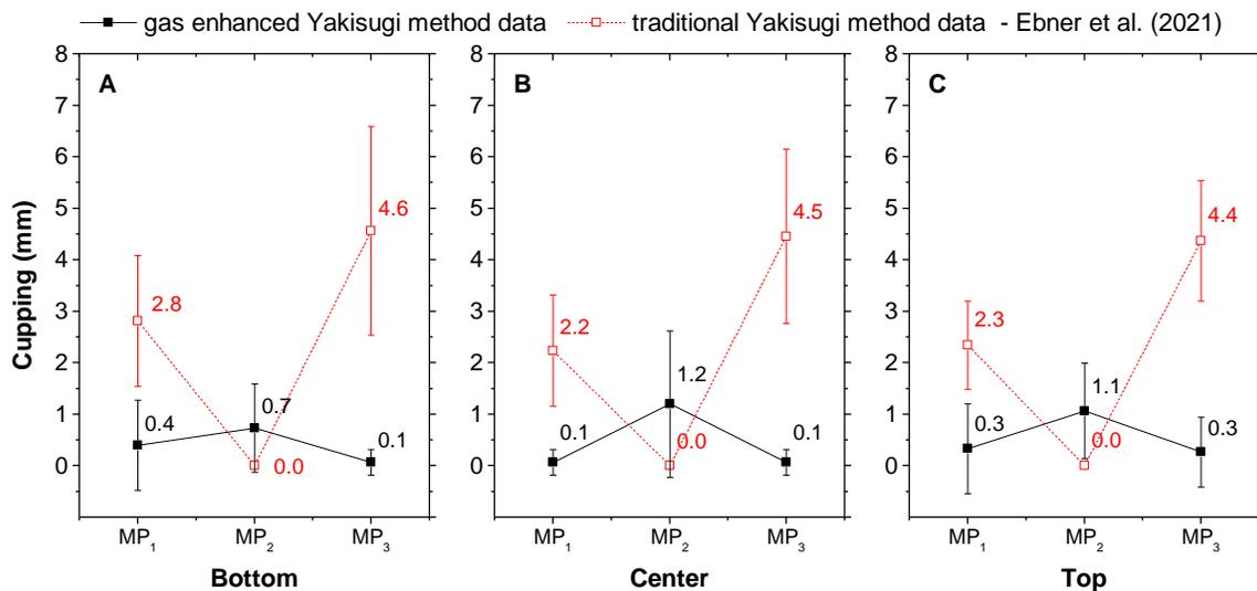
**Fig. 6.** The cupping at: cut line 1 – bottom (A); cut line 2 – middle (B); and cut line 3 - top (C)
