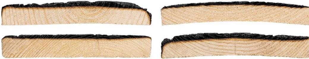
**Fig. 7.** Visual comparison of boards showing the varied charred layer thickness and cupping effect
