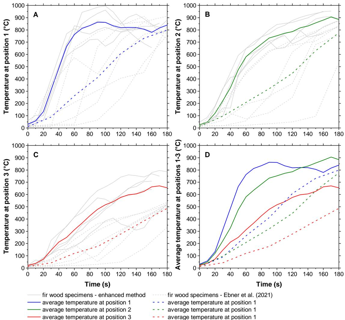
**Fig. 3.** Temperature-time diagram for the fir samples measured at positions 1, 2 and 3 (A through C) and the average temperature data (D). Solid line depicts values obtained by enhanced method, while dotted line stands for values recorded by Ebner *et al.* (2021).
