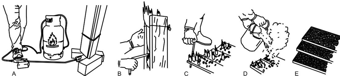
**Fig. 1.** The methodology of one-sided surface charring *via* the traditional Japanese yakisugi technique enhanced with propane gas ignition
