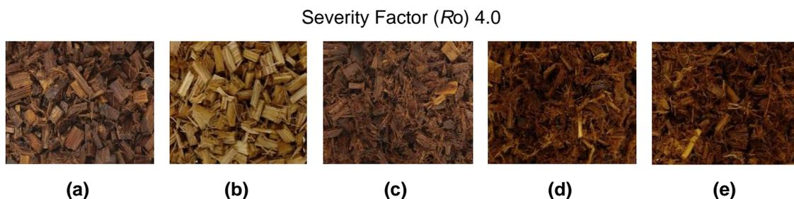
**Fig. 2.** Images of the pine chips obtained from different steam explosion conditions at the same severity factor ( $R_o$ ) of 4.0: (a) 190 °C, 20.0 min; (b) 200 °C, 11.5 min; (c) 210 °C, 6.0 min; and (d) 220 °C, 3.0 min; (e) 230 °C, 1.5 min
