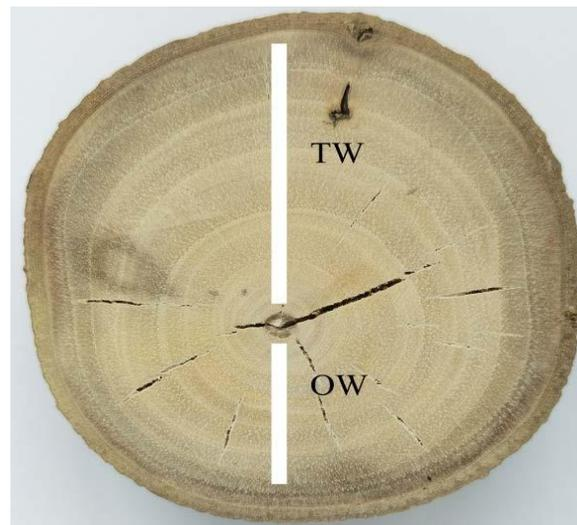
**Fig. 1.** The selection process of samples containing tension wood (TW) and opposite wood (OW)
