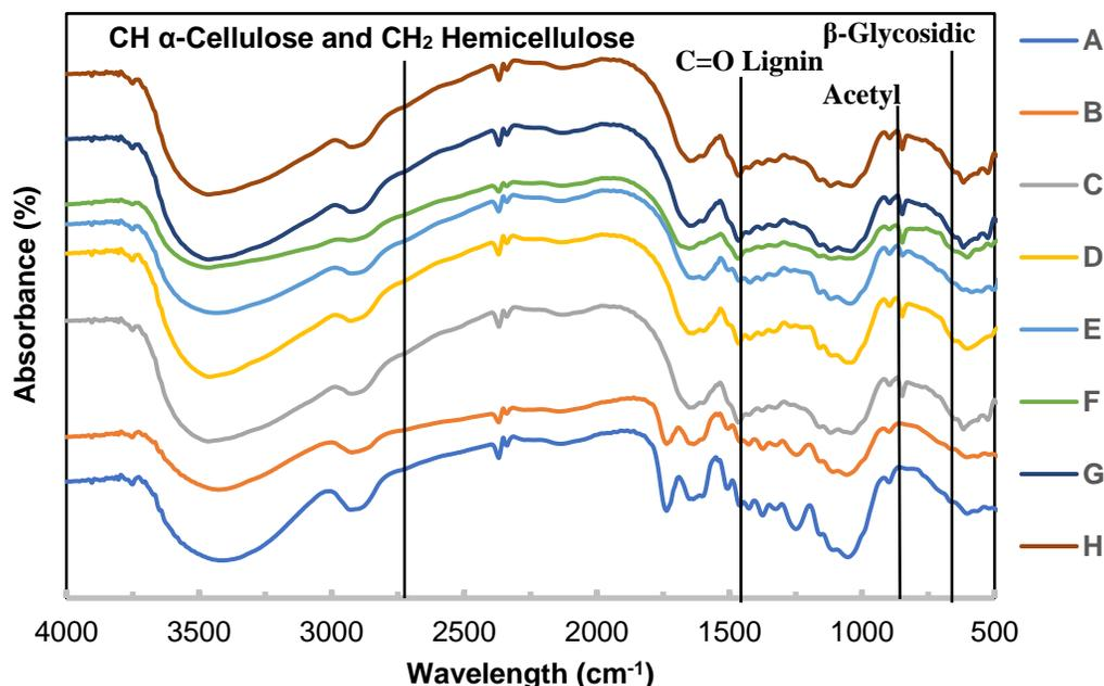
**Fig. 1.** FTIR spectra of modified FVB (Note: A. Untreated for 30 min; B. untreated for 60 min; C. 1% NaOH for 30 min; D. 1% NaOH for 60 min; E. 1% NaOH + 0.2% Na<sub>2</sub>SO<sub>3</sub> for 30 min; F. 1% NaOH + 0.2% Na<sub>2</sub>SO<sub>3</sub> for 60 min; G. 1% NaOH + 0.4% Na<sub>2</sub>SO<sub>3</sub> for 30 min; and H. 1% NaOH + 0.4% Na<sub>2</sub>SO<sub>3</sub> for 60 min)
