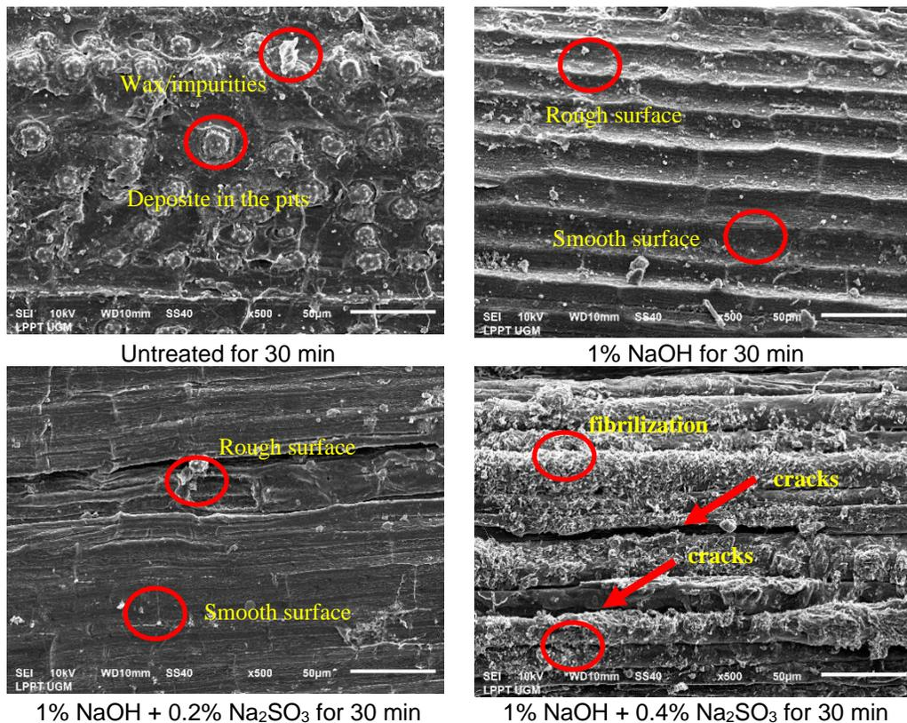
**Fig. 3.** Surface morphology of the modified FVB from *S. sumatrana* fronds
