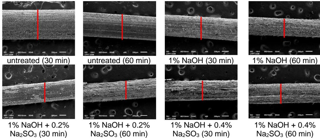
**Fig. 2.** SEM images of the modified FVB. The diameters are indicated by the red bar.
