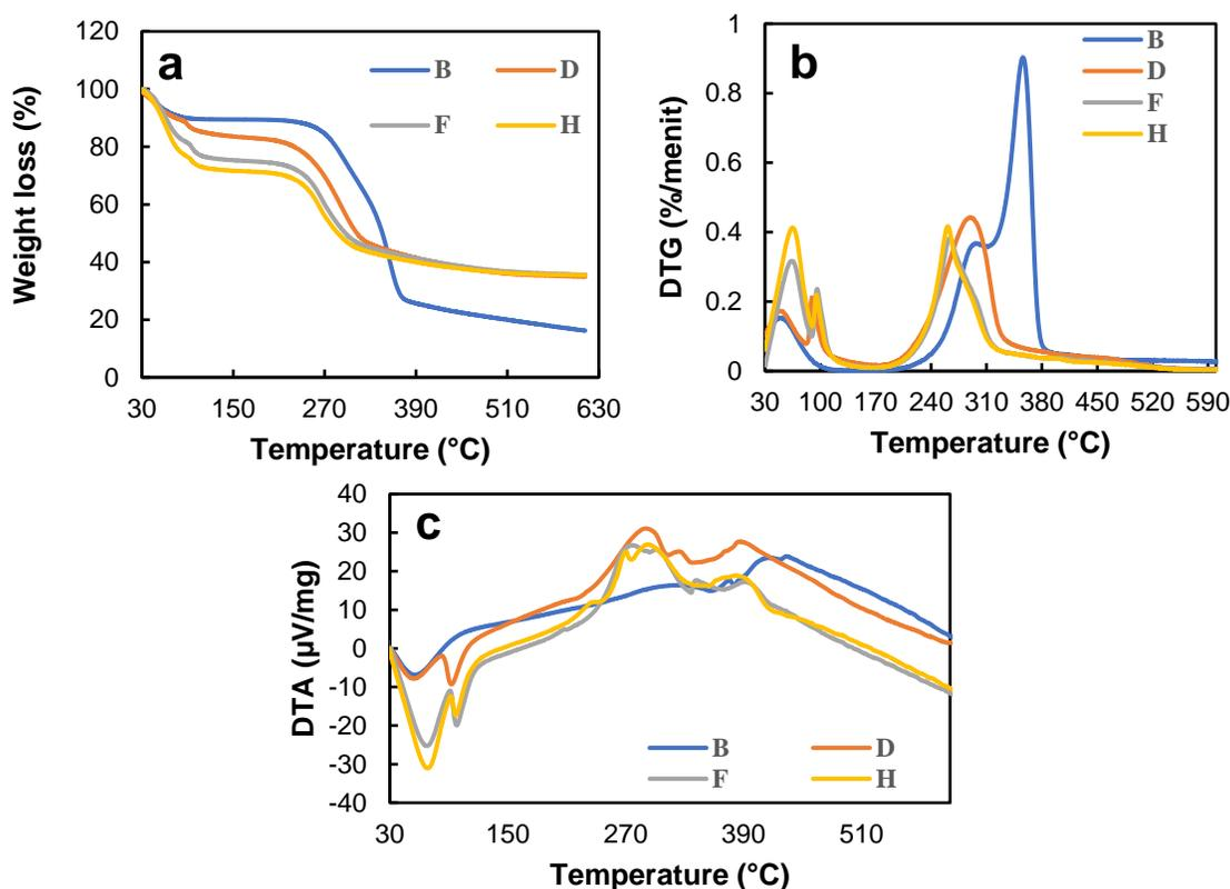
**Fig. 6.** The thermogram of (a) reduction in weight; (b) DTG; and (c) DTA (Note: B. untreated for 60 min; D. 1% NaOH for 60 min; F. 1% NaOH + 0.2% Na<sub>2</sub>SO<sub>3</sub> for 60 min; and H. 1% NaOH + 0.4% Na<sub>2</sub>SO<sub>3</sub> for 60 min)
