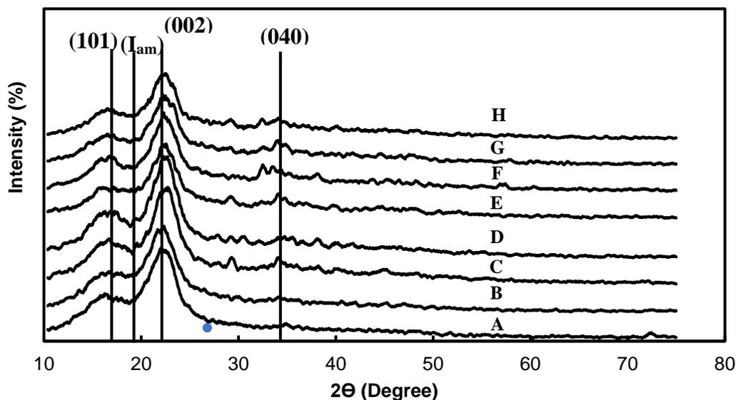
**Fig. 5.** XRD diffractogram of modified FVB from *S. sumatrana* fronds (Note: A. Untreated for 30 min; B. untreated for 60 min; C. 1% NaOH for 30 min; D. 1% NaOH for 60 min; E. 1% NaOH + 0.2% Na<sub>2</sub>SO<sub>3</sub> for 30 min; F. 1% NaOH + 0.2% Na<sub>2</sub>SO<sub>3</sub> for 60 min; G. 1% NaOH + 0.4% Na<sub>2</sub>SO<sub>3</sub> for 30 min; and H. 1% NaOH + 0.4% Na<sub>2</sub>SO<sub>3</sub> for 60 min)
