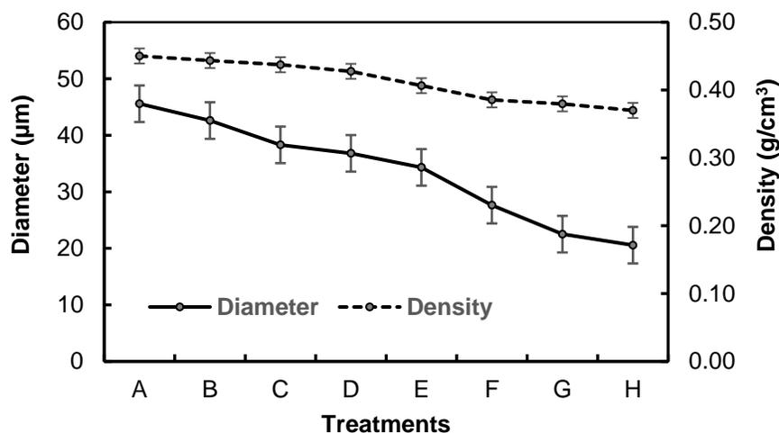
**Fig. 4.** The diameter and density of the modified fibrovascular bundles (Note: A. Untreated for 30 min; B. untreated for 60 min; C. 1% NaOH for 30 min; D. 1% NaOH for 60 min; E. 1% NaOH + 0.2%  $\text{Na}_2\text{SO}_3$  for 30 min; F. 1% NaOH + 0.2%  $\text{Na}_2\text{SO}_3$  for 60 min; G. 1% NaOH + 0.4%  $\text{Na}_2\text{SO}_3$  for 30 min; and H. 1% NaOH + 0.4%  $\text{Na}_2\text{SO}_3$  for 60 min; in addition, the vertical bars indicate the standard deviation)
