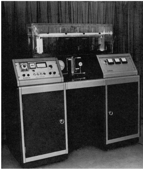
Fig. 6 —Photograph of a commercial version of the large volume microwave plasma generator
