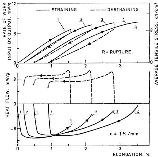
**Fig. 6**—Thermodynamic behaviour of plasticised regenerated cellulose film CD during successive load/elongation cycles
