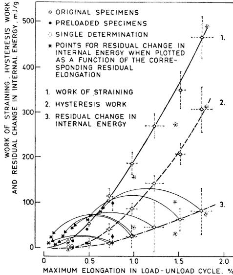
**Fig. 10**—Work of straining, hysteresis work and residual change in internal energy as functions of maximum elongation in load/unload cycle for 100 per cent rag paper CD
