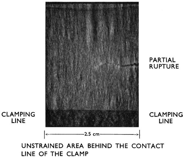
**Fig. 11**—Partially ruptured tensile specimen of handsheet  $B_m$
