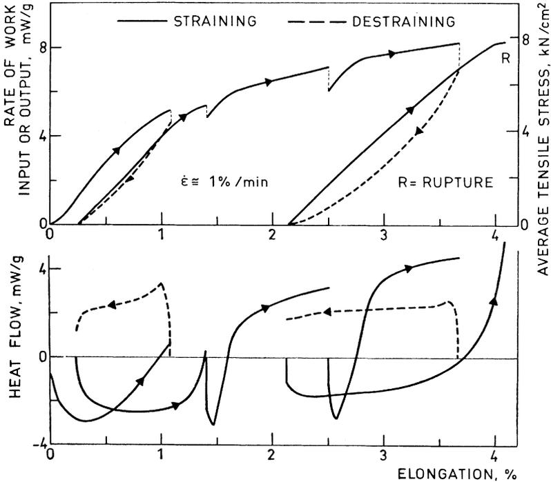
Fig. 3—Thermodynamic behaviour of clupak sackpaper MD
