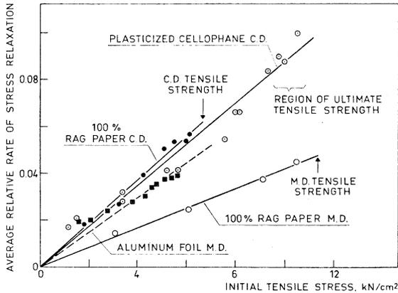
Fig. 8—Refined stress relaxation data for rag paper, regenerated cellulose film and aluminium
