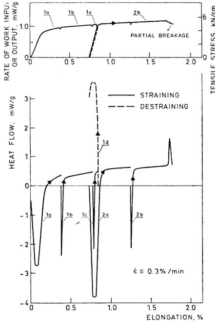
**Fig. 7**—Thermodynamic behaviour of aluminium foil MD
