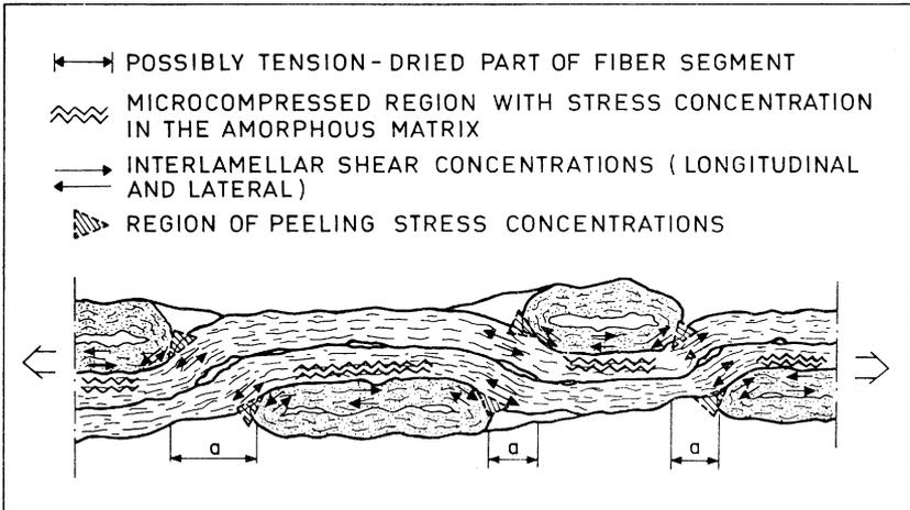
**Fig. 12**—Schematic representation of some possible stress concentration regions in apparent plastic straining of paper
