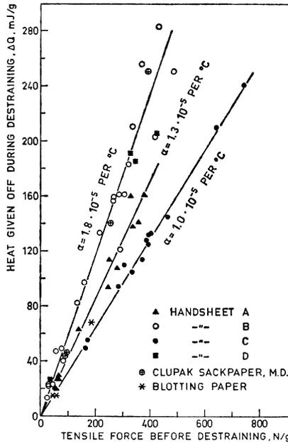
**Fig. 9**—Relationship between heat output and tensile force in destaining runs of different handsheets and miscellaneous papers
