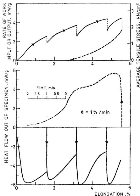
**Fig. 5**—Thermodynamic behaviour of spunbonded polyolefin paper
