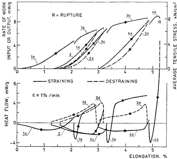
Fig. 4—Thermodynamic behaviour of handsheet D
