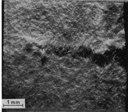
ENLARGEMENT OF A TYPICAL RUPTURE LINE
