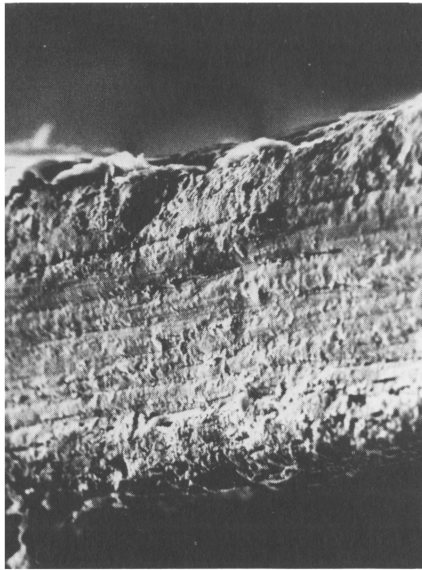
Fig. 13 —Section of 'second generation' plastics paper (Magnification \times 700 )
