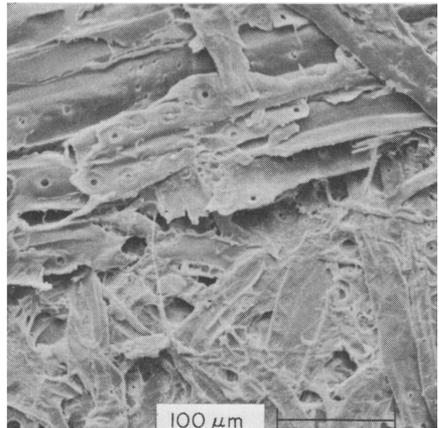
**Fig. 20**—Delamination in newsprint flexed 80 000 times over 3·18 mm rollers  $\times 225$
