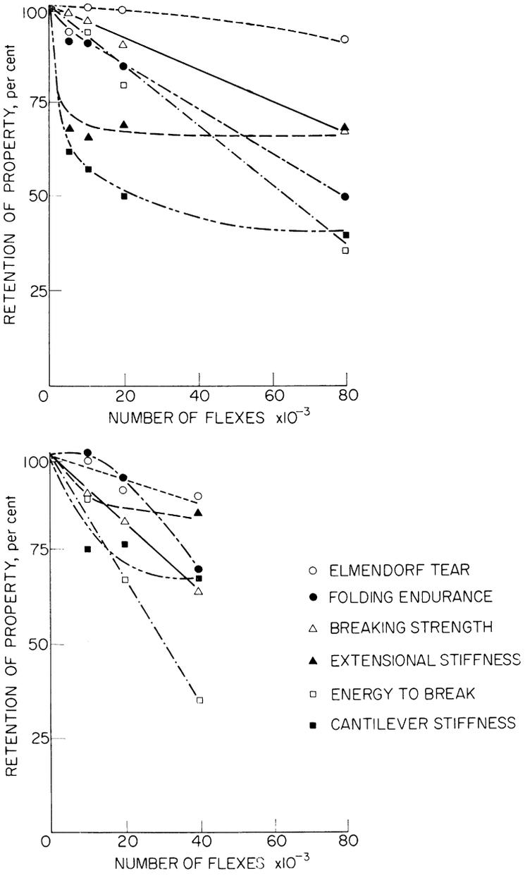
Fig. 5—Degradation of physical properties of high grade rag paper during flexing
