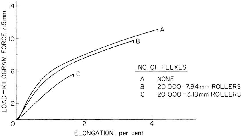
Fig. 12—Effect of roller size on the load/elongation properties of high grade rag paper when flexed in the MD
