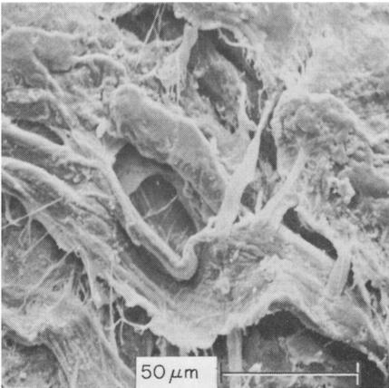
**Fig. 19**—Delamination in all cotton ledger paper flexed 80 000 times over 3·18 mm rollers  $\times 595$
