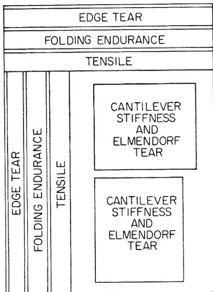
Fig. 3—Specimen layout for flexed samples
