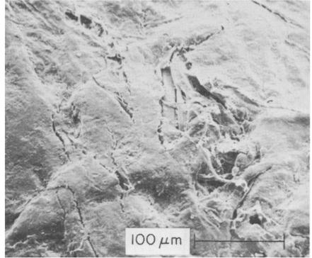
**Fig. 21**—Cracks running in both CD and MD after flexing in CD over 3.18 mm rollers  $\times 860$
