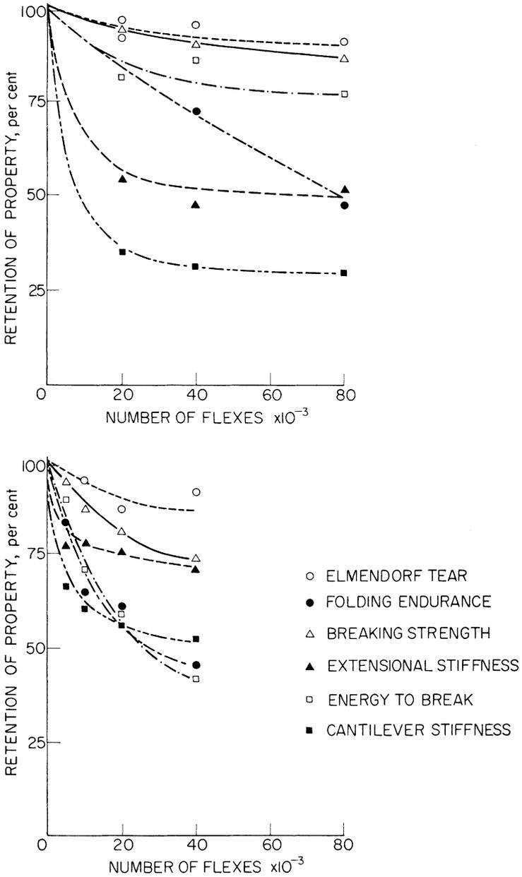
Fig. 6—Degradation of physical properties of cotton ledger paper during flexing
