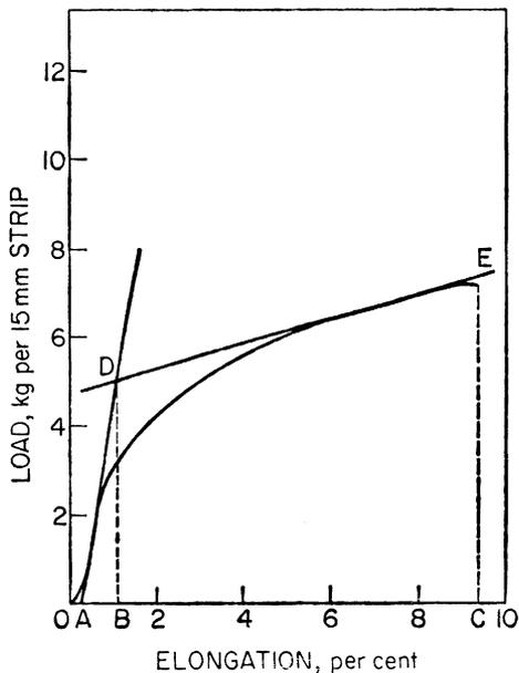
Fig. 4—Typical load/elongation curve for paper
