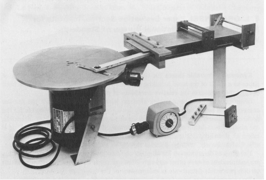
*Fig. 1*—Paper flexing apparatus
