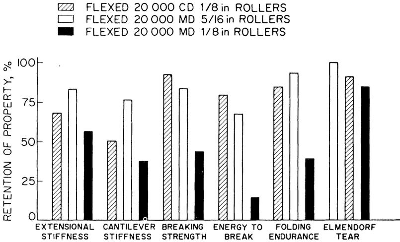
Fig. 11—Effect of strain level during flexing on the degradation of physical properties
