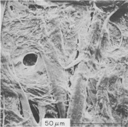
**Fig. 17**—All cotton ledger paper flexed 80 000 times in CD over 3·18 mm rollers: cracks are running parallel to MD  $\times 660$
