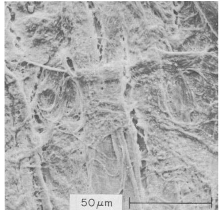
**Fig. 16**—High grade rag paper flexed 80 000 times in CD over 3·18 mm rollers: cracks are running parallel to MD  $\times 650$
