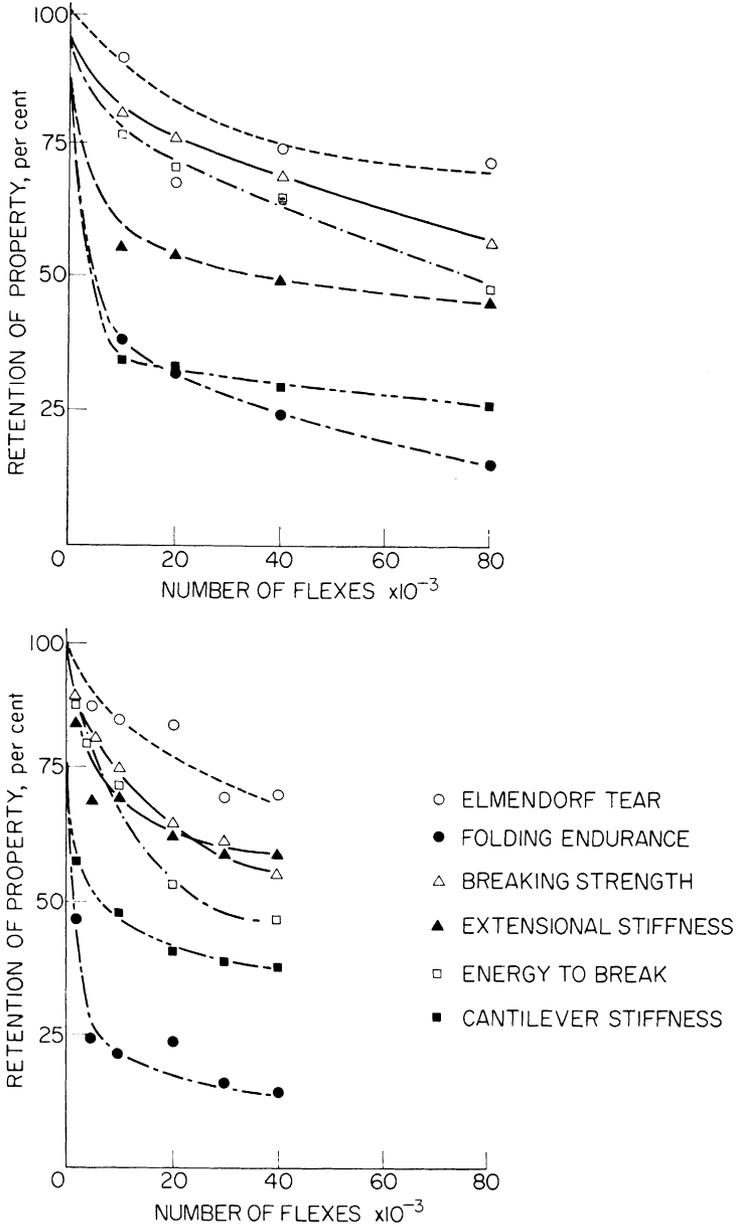
Fig. 7—Degradation of physical properties of newsprint during flexing
