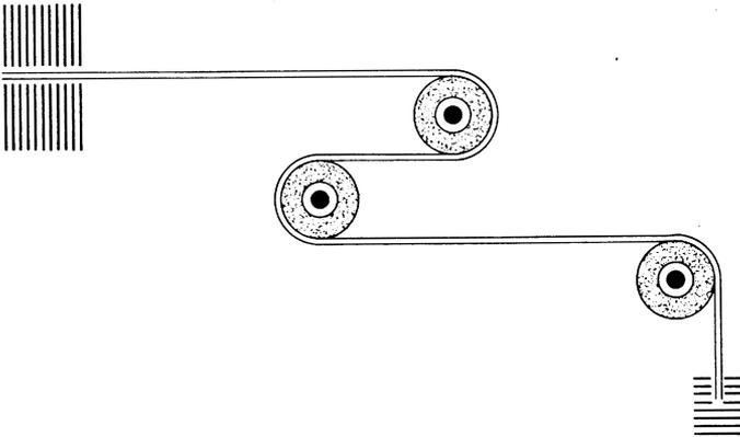
*Fig. 2*—Schematic diagram for paper flexing
