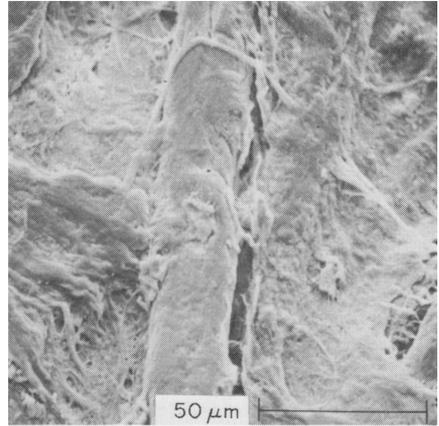
**Fig. 18**—Newsprint flexed 80 000 times in CD over 3·18 mm rollers: cracks are running parallel to MD  $\times 660$
