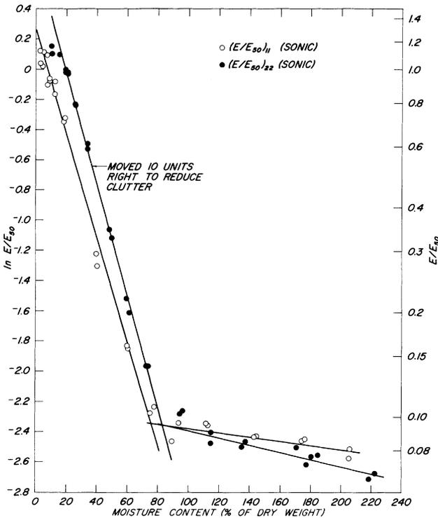
Fig. 5—Dependence of sonic modulus on moisture for uncrosslinked kraft linerboard in machine and cross-machine direction
