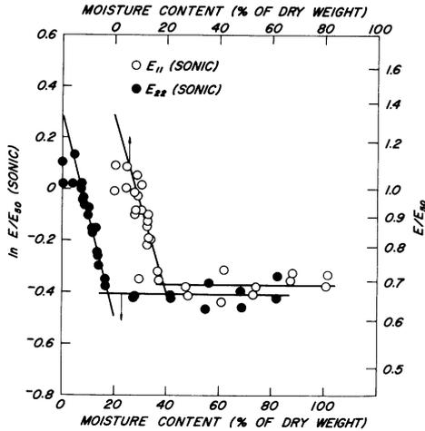
Fig. 6—Dependence of sonic modulus on moisture for crosslinked kraft linerboard in machine and cross-machine direction
