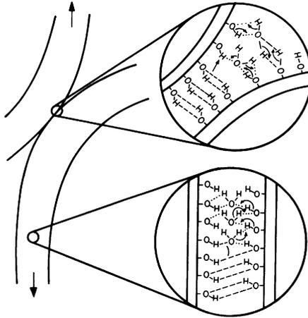
**Fig. 2**—Two wet cellulose fibrils. Hydrogen-bonded array may flicker more easily into new configuration of bonds, in which some bonds are stress relaxed. A greater strain is experienced by those bonds that do not relax
