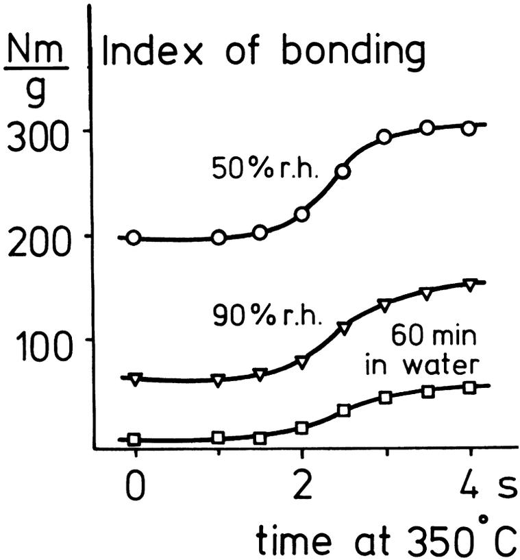
*Fig. 2*—The Page bonding index of unbleached kraft paper in the moist and wet state as a function of heating period at 350° C employed to cause auto-crosslinking. Data by E. Stenberg (2)
