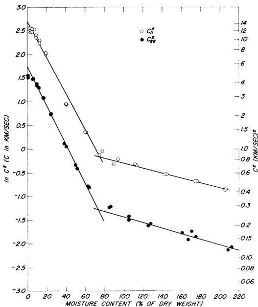
**Fig. 3**—Dependence of sonic velocity on moisture for uncrosslinked kraft linerboard in the machine and cross-machine direction
