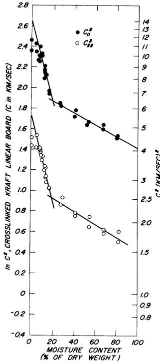
**Fig. 4**—Dependence of sonic velocity on moisture for crosslinked kraft linerboard in machine and cross-machine direction
