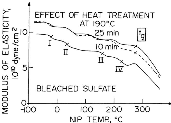
**Fig. 1**—Modulus of elasticity in the dry (water free) state of untreated and auto-crosslinked paper of bleached kraft as a function of uncorrected temperatures (1)
