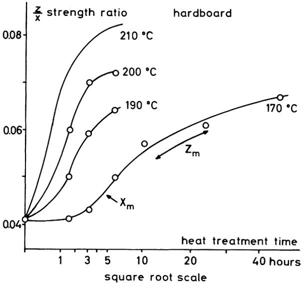
**Fig. 3**—The strength ratio in the  $z$ - to  $x$ -direction (perpendicular to sheet relative machine direction) for hardboard of a thermo-mechanical pulp without a resin binder. The strength ratio is given versus the heat treatment time at a few commercially used temperatures (3)
