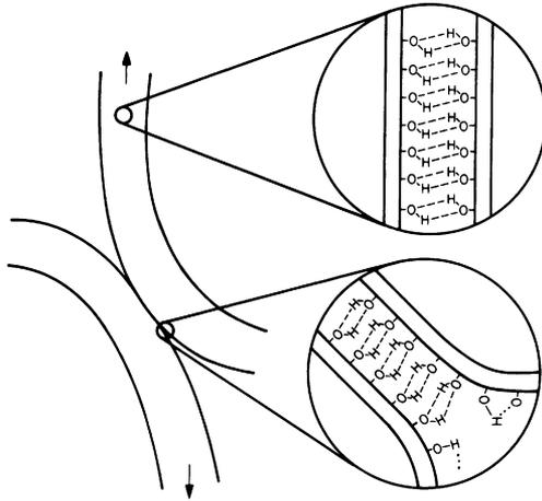
**Fig. 1**—Schematic of two cellulosic fibrils in contact, showing hydrogen-bonded nature in the interfibre region and within the cell wall
