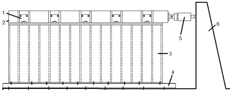
1. Cantilever load transfer device; 2. Load transfer beam; 3. LVL shear wall; 4. Base steel beam; 5. FTS hydraulic servo system; 6. Reaction wall
