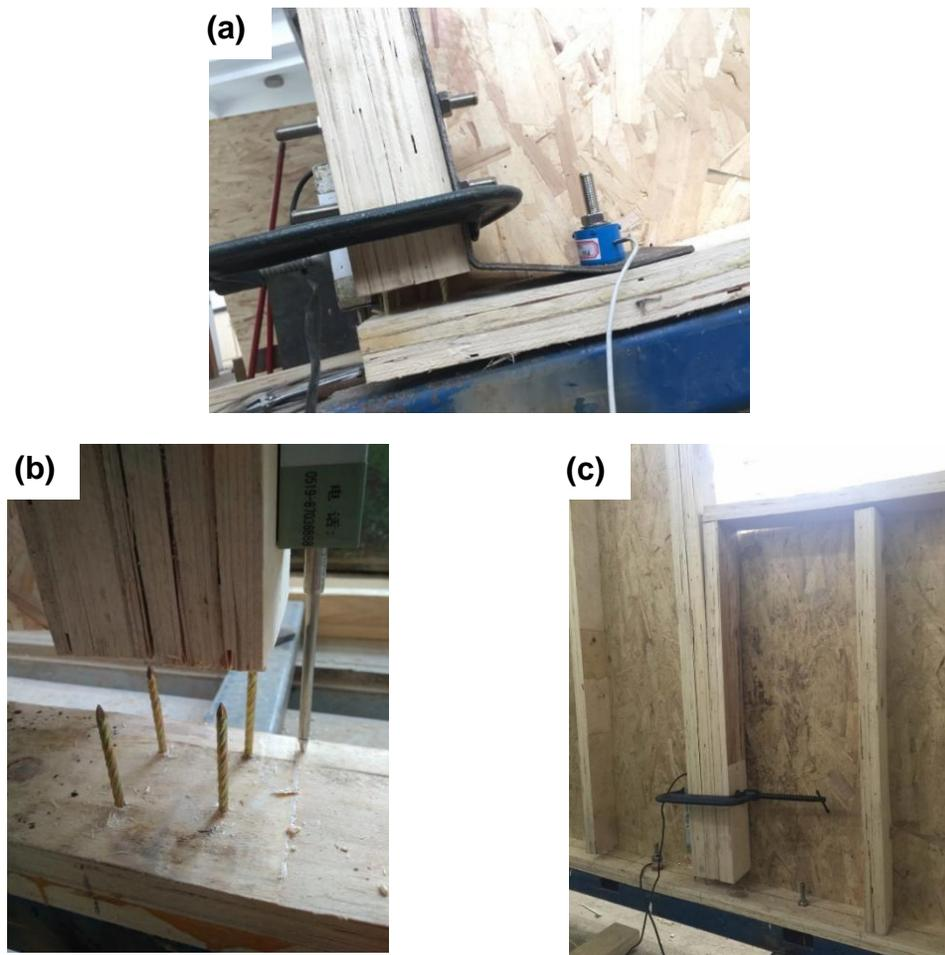
Fig. 8. Separation between the studs and the base plate (a) Wall-A; (b) Wall-B; (c) Wall-C
