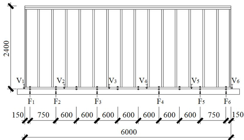
**Fig. 4.** Layout of the measuring points (unit: mm)
