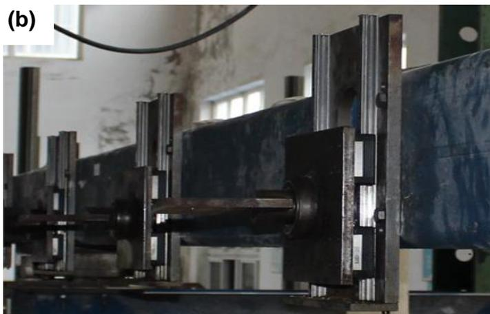
(b) Cantilever load transfer device
