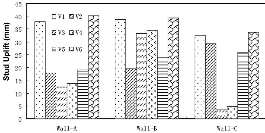
Fig. 9. The maximal separation distance between the studs and the base plate for cyclic test by Guo (2010)
