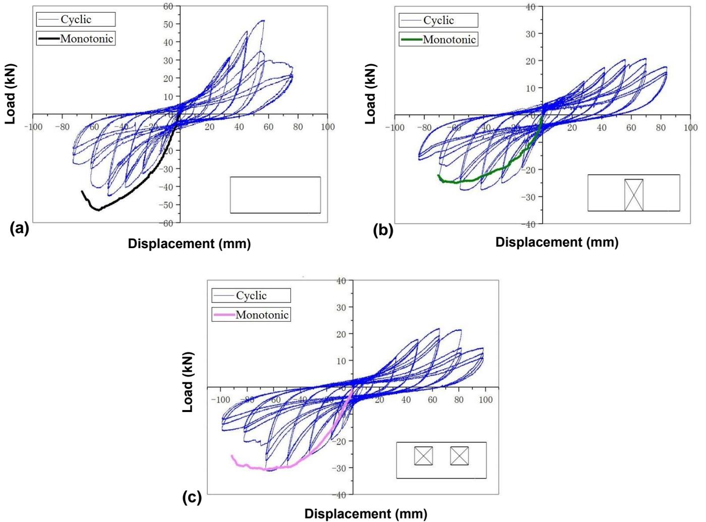
Fig. 10. The load-displacement curve: (a) wall A; (b) wall B; (c) wall C
