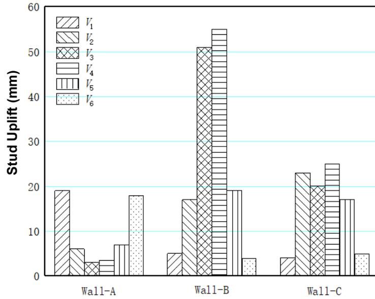
Fig. 7. The maximal separation distance between the studs and the base plate in cyclic test
