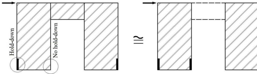
Fig. 13. The calculation guidance for shear-wall limbs with only one hold-down
