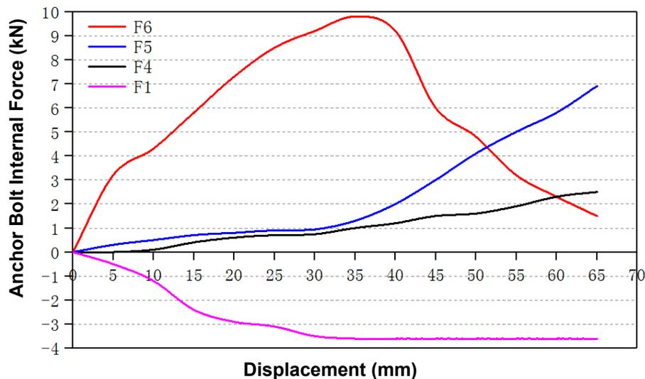
**Fig. 11.** The internal force of the base plate anchor bolts of the Wall-A specimen
