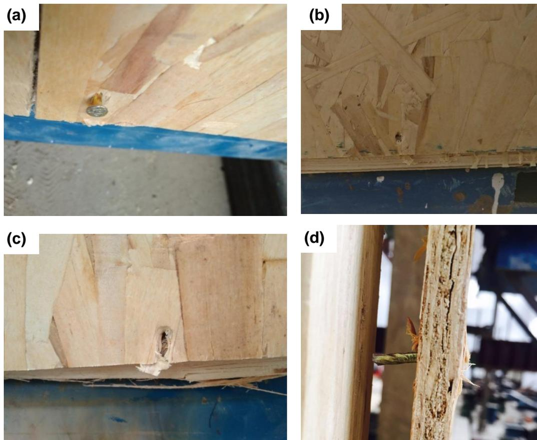
(a) Bottom nail was pulled out; (b) Bottom nail head penetrated the panel; (c) Bottom panel edge was torn; (d) Side nail was sheared to fracture due to fatigue
