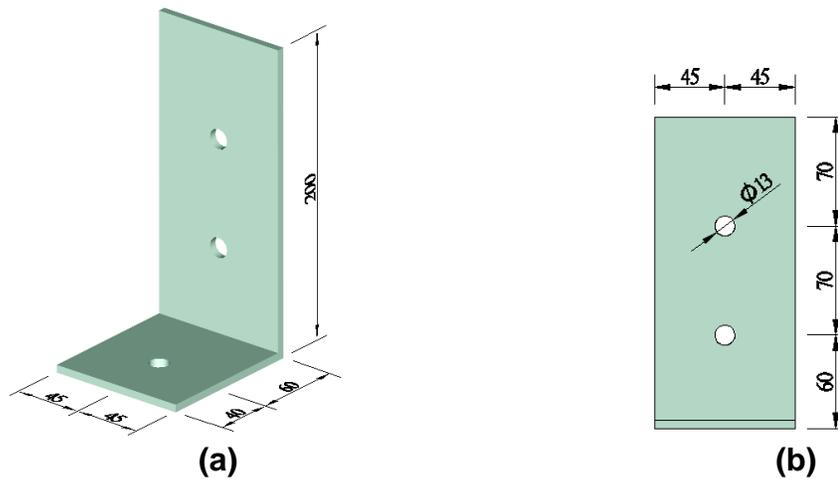
**Fig. 2.** The details of the custom-designed hold-down (unit: mm). (a) Perspective; (b) side view
