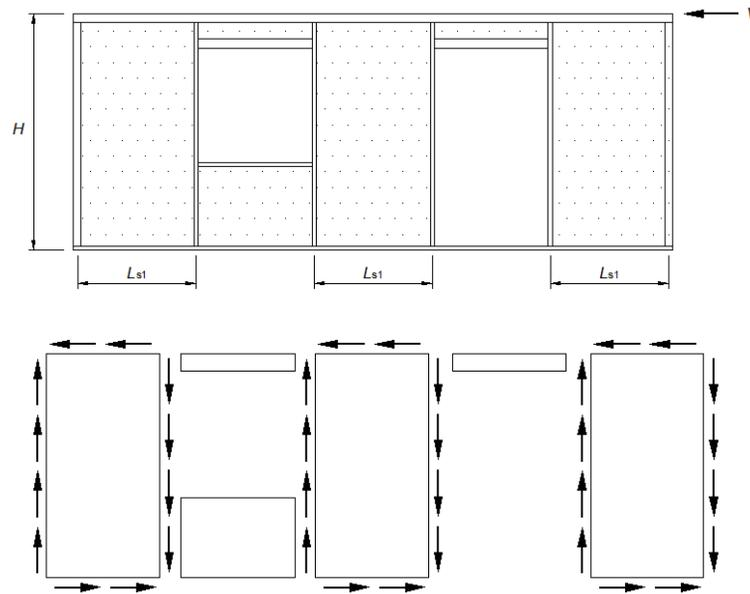
**Fig. 12.** The schematic diagram for calculation of the shear wall bearing capacity
