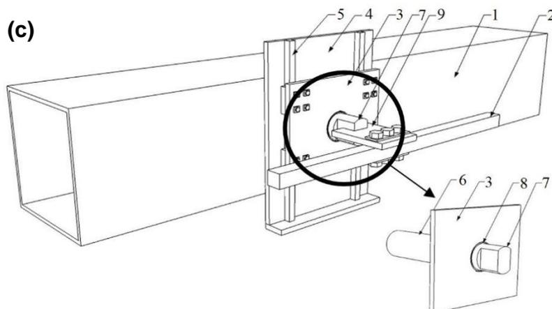
1. Square steel tube; 2. Top plate; 3. Inner steel plate; 4. Outer steel plate; 5. Slide rail; 6. Steel pipe; 7. Steel rod; 8. Bearing; 9. Center steel plate
